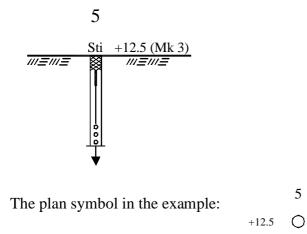
Presented without showing the penetration resistance. Estimated soil type on the basis of the sounding result can be shown. In this case the grade of observation Mk3 (see appendix 1) has been applied.
