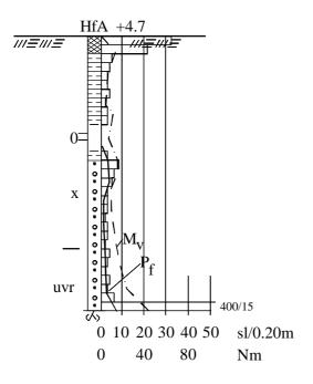
Is carried out according to method A or B. The penetration resistance is noted as the number of blows required per 0.2 m of penetration (sl/0.2 m) and is presented in a bar chart. Different scales can be used. The turning resistance ( $M_v$  in Nm) and calculated frictional resistance ( $P_f$  in sl/0.2 m) can be left out. Estimated soil types in connection with the sounding operation can be noted in the borehole column.
