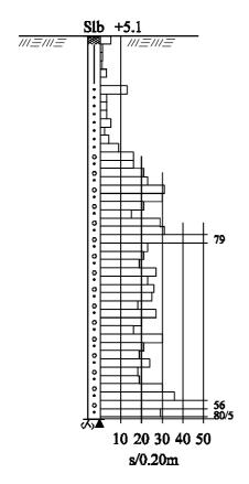
The resistance is shown as penetration time per depth interval (sec./0.2 m) and is presented in a bar chart.
