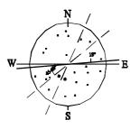
Presentation of fractures in a so-called stereo net (Schmidt diagram). The plan of the fracture is shown with a point, the pole of which is a projection of the point where a normal to the plan intersects the lower hemisphere. The observations can be brought together to form interpreted main directions represented by the broken lines in the fracture diagram.
