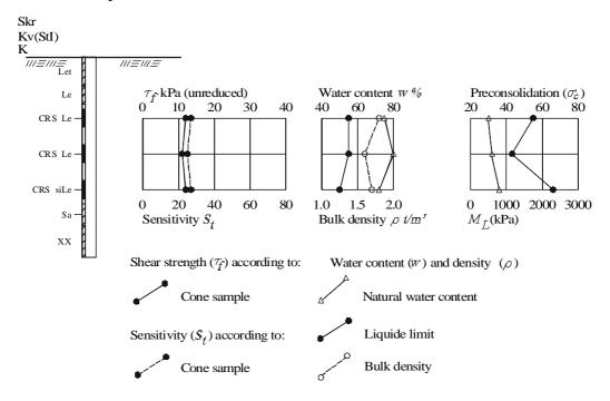
In the diagrams are presented uncorrected shear strength ( $t_k$ ) and sensitivity ( $S_{tk}$ ), water contents (natural  $w_N$ , liquid limit  $w_L$ ) and bulk density (r), preconsolidation pressure ( $s'_c$ ) and compression modulus  $M_L$ , determined by means of oedometer tests, in this case CRS tests.
