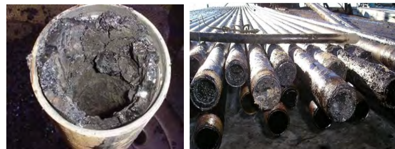
Plugging in the wellbore
