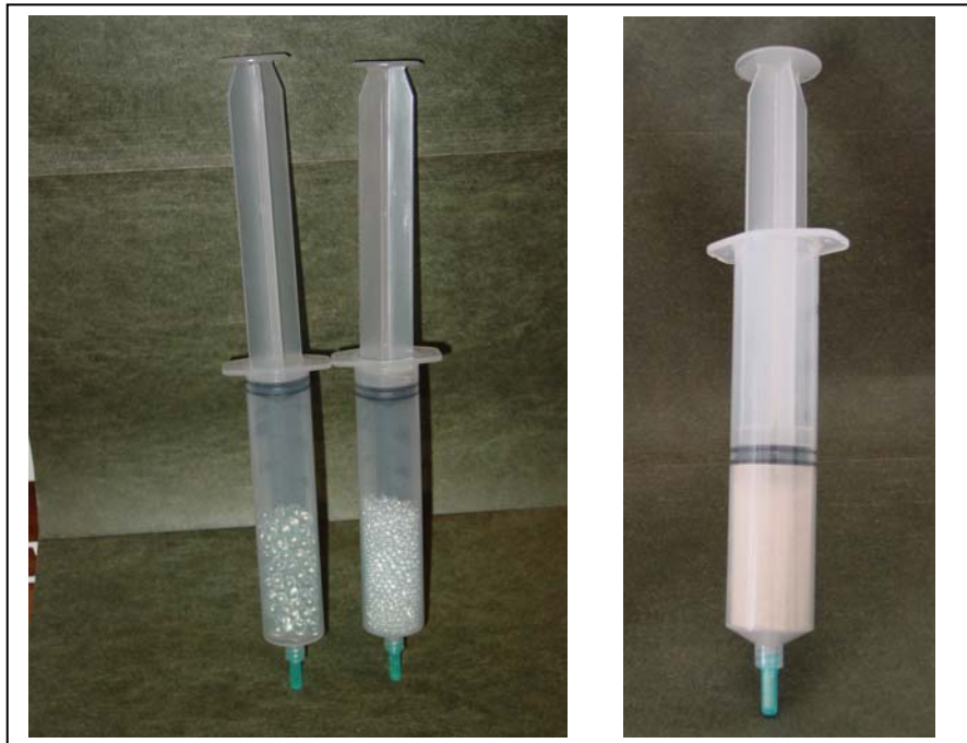
Figure 2. Left picture demonstrates experiment with glass beads as an alternative approach to two different sized sands. The second picture on the right demonstrates the syringe with fine sand.
