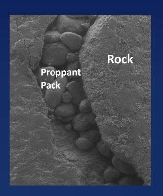
$$C_{fD} = {Frac Conductivity} = {W \times k_{frac-retained}} = {X_L \times k_{formation}}$$
