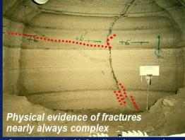
Source: Warpinski, Sandia Labs. Nevada Test Site, Hydraulic Fracture Mineback
