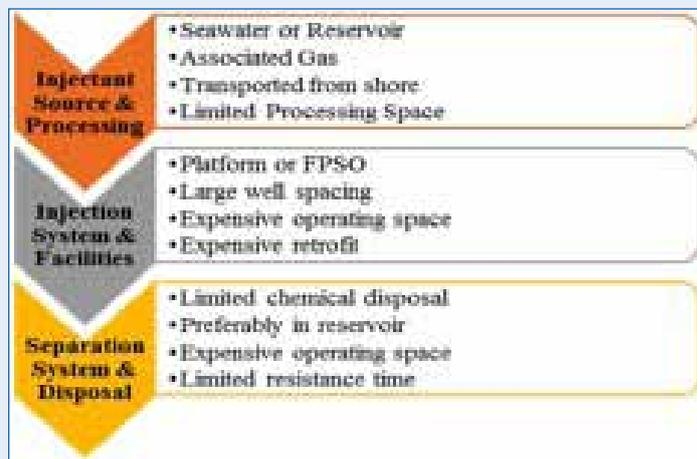
**Figure 3 (above):** Challenges associated with implementation and post-production facilities required (Alvarado,V et al., 2013)
