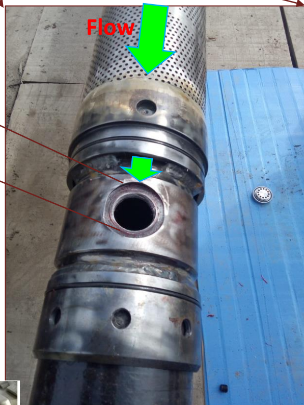
Autonomous Inflow Control Devices AICD 7.5 mm
