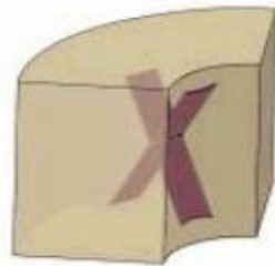
Shear Failure Shallow Knockout (Ssko)
