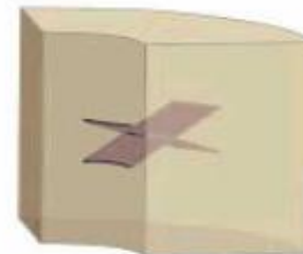
Shear Failure Deep Knockout (Sdko)
