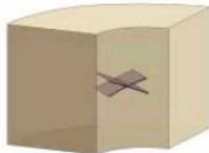
Shear Failure Low Angle Echelon (Slae)
