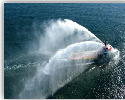
AHTS water spray systems in operation
