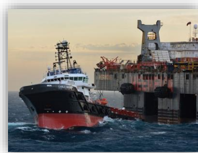
Inclusive in bad conditions of the sea, de DP II will maintain the position
