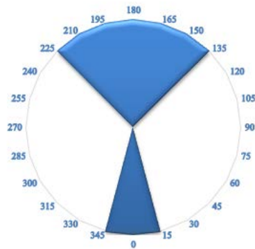
Stationkeeping at Sea State 4, 0.5kts Current: 500 kW Bow Thruster Effectiveness
