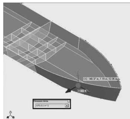
**Figure 6.** The “Measure Area” tool can be used to calculate the area of a boat hull plate, including curved surfaces, quickly and easily. The Center of Gravity feature of Inventor can be used to obtain values for all three centers of gravity—transversal, vertical, and longitudinal—for a boat hull plate. These values can then be entered into the spreadsheet by the students.
