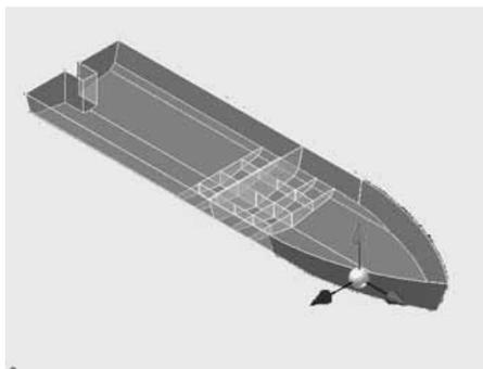
**Figure 4.** The "Derived Component" feature of Inventor can be used to produce a "Phantom" boat or a boat without physical properties (shown here by middle part of the structure). The "Thicken" tool is used to give a plate some physical properties, shown by the shaded area. A work surface is shown with one curved plate "thickened" and its associated center of gravity.
