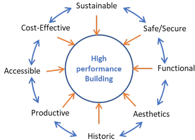
Fig. 8. Overview of the connection between the design objectives as defined by the WBDG and the development of a high-performance building.
