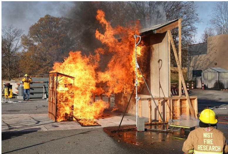
Fig. 2. A full-scale outdoor shed experiment with applied wind field.
