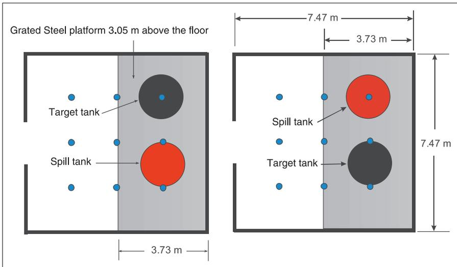
**Figure 5.** The layout of ceiling nozzles, storage tanks and grated steel platform in the full-scale building.
