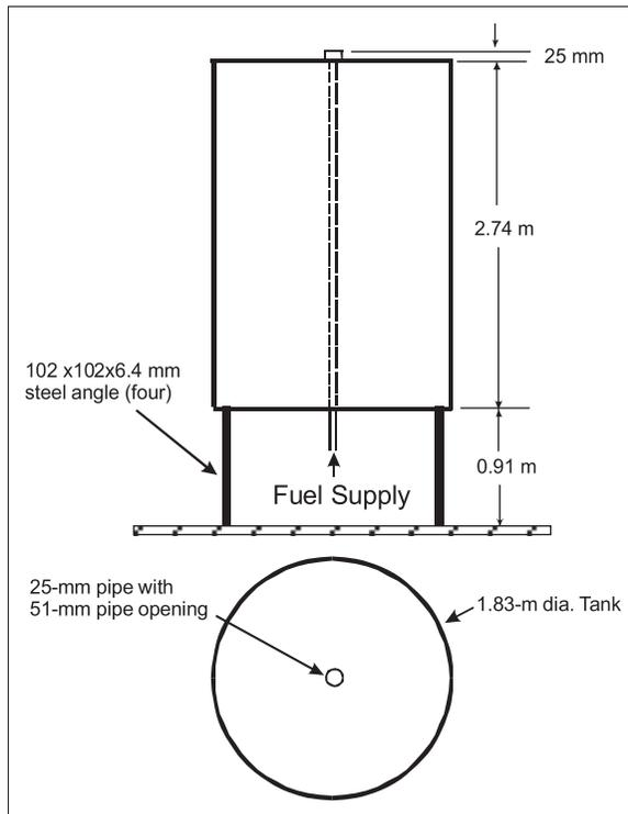
**Figure 3.** A schematic of the ignitable liquid storage tank mockup.
