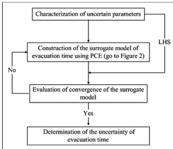
**Figure 1.** Flowchart of the iterative procedure for quantifying evacuation time uncertainty using polynomial chaos expansion (PCE).
