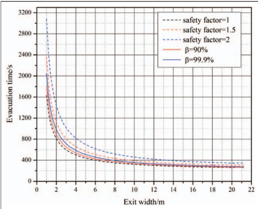
Figure 5. The relationship between evacuation time and exit width.
