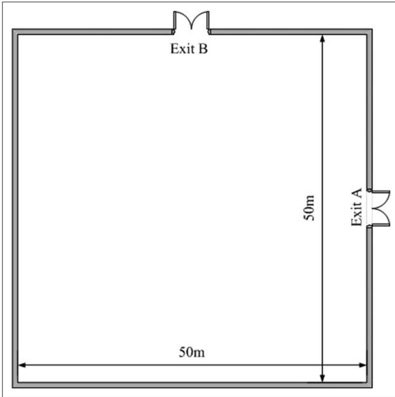
**Figure 3.** A simplified fire compartment for commercial buildings.
