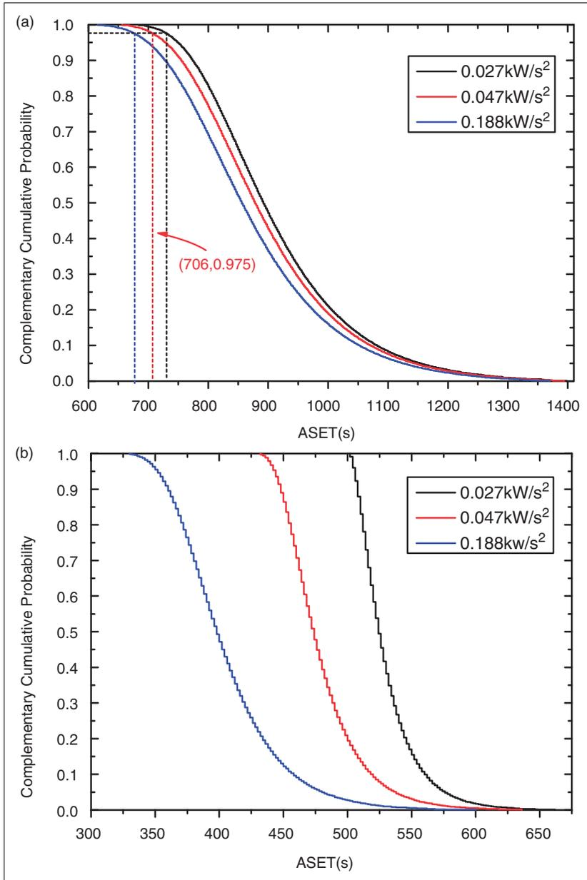
**Figure 6.** Complementary cumulative distribution of predicted ASET with normal distribution of peak HRR for three kinds of fire growth rate: (a) normal peak HRR with a mean of 2000 kW; (b) normal peak HRR with a mean of 5500 kW. ASET: available safe egress time; HRR: heat release rate.
