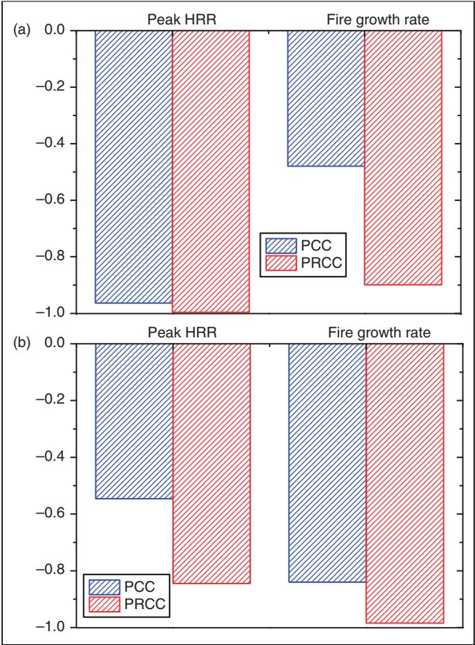
**Figure 10.** Sensitivity results based on PCC and PRCC for the predicted ASET: (a) normal peak HRR with a mean of 2000 kW and log-normal fire growth rate; (b) normal peak HRR with a mean of 5500 kW and log-normal fire growth rate. ASET: available safe egress time; HRR: heat release rate; PCC: partial correlation coefficient; PRCC: partial rank correlation coefficient.
