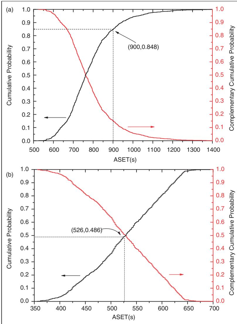
**Figure 9.** Cumulative probability curve and complementary cumulative probability curve of predicted ASET: (a) normal peak HRR with a mean of 2000 kW and log-normal fire growth rate; (b) normal peak HRR with a mean of 5500 kW and log-normal fire growth rate. ASET: available safe egress time; HRR: heat release rate.
