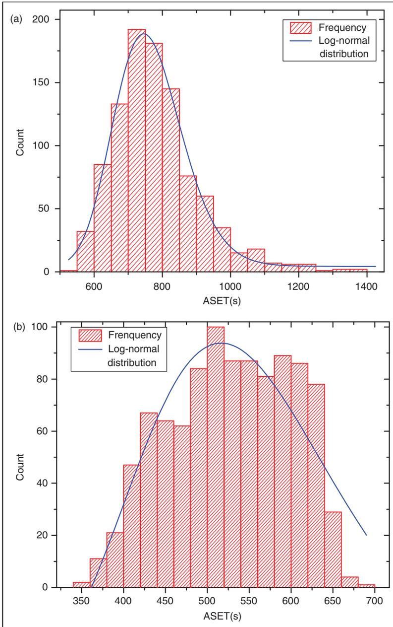
**Figure 8.** Probability distribution of predicted ASET and theoretical log-normal distribution curve fit: (a) normal peak HRR with a mean of 2000 kW and log-normal fire growth rate; (b) normal peak HRR with a mean of 5500 kW and log-normal fire growth rate.
