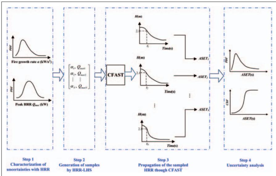
**Figure 2.** Schematic of uncertainty analysis for ASET. ASET: available safe egress time.
