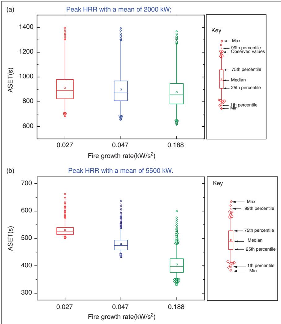
**Figure 5.** Box plot of predicted ASET with normal distribution of peak HRR and deterministic fire growth rates: (a) normal peak HRR with a mean of 2000 kW; (b) normal peak HRR with a mean of 5500 kW.
