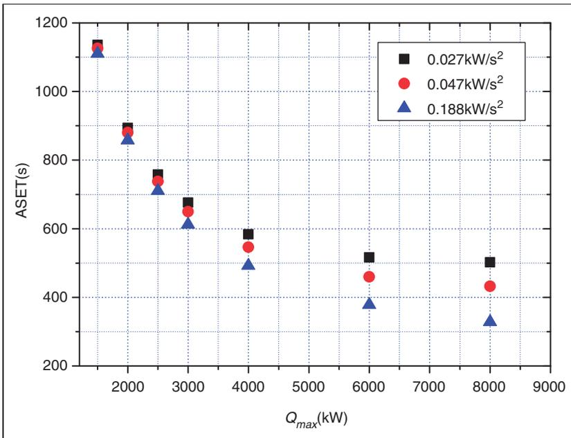
**Figure 4.** ASET calculated by deterministic peak HRR and fire growth rate. ASET: available safe egress time; HRR: heat release rate.
