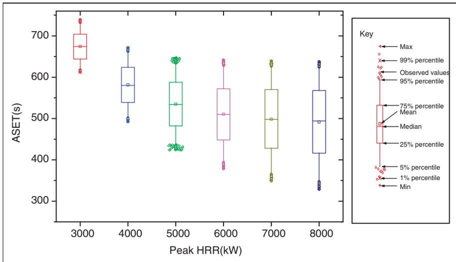
**Figure 7.** Box plot of the predicted ASET with six different peak HRRs. ASET: available safe egress time; HRR: heat release rate.
