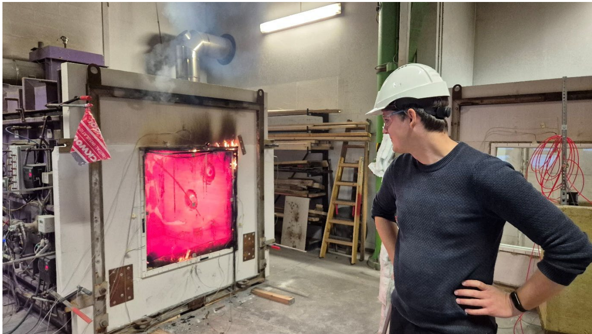
Figure 1. Picture from one of the tests showing a hot window in the furnace.
