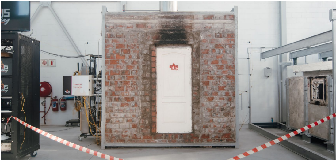
Figure 1: Vertical furnace and SCADA system at Ignis Testing
