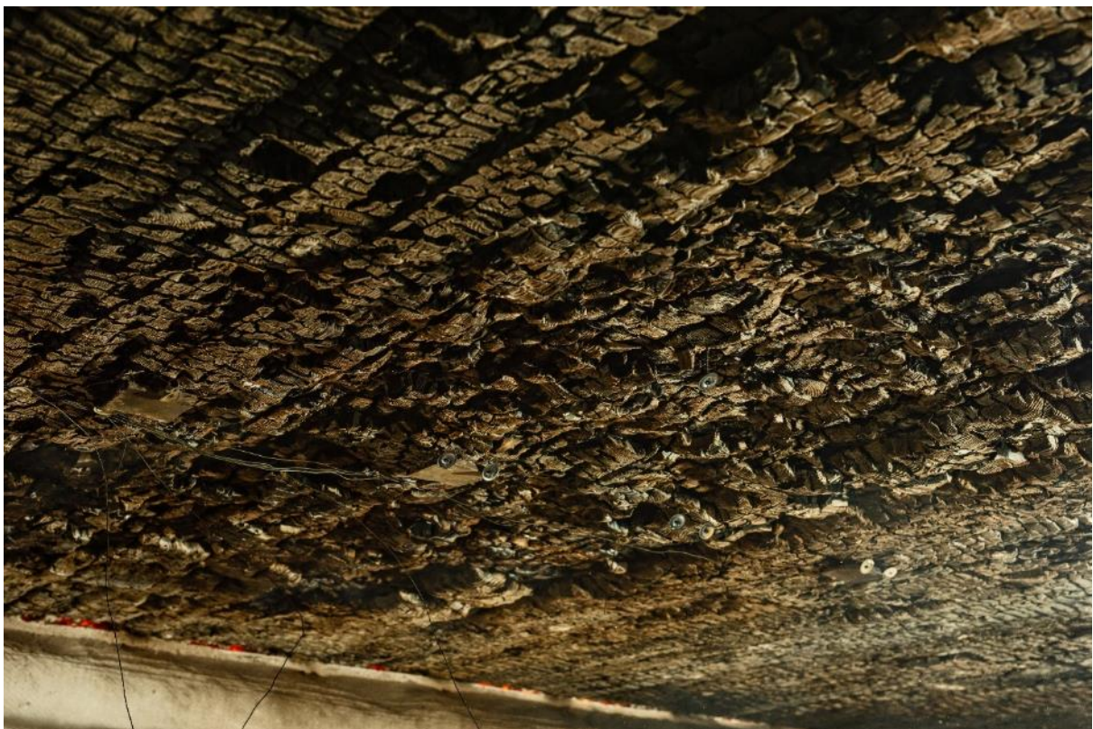
Figure 5. Extensive GLIF in vicinity of burner in experiment 2.
