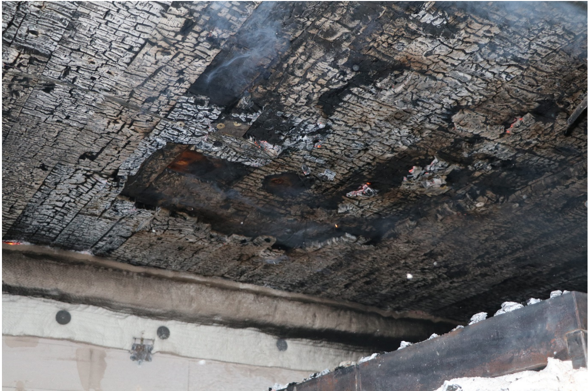
Figure 5. Extensive GLIF in vicinity of burner in experiment 2.
