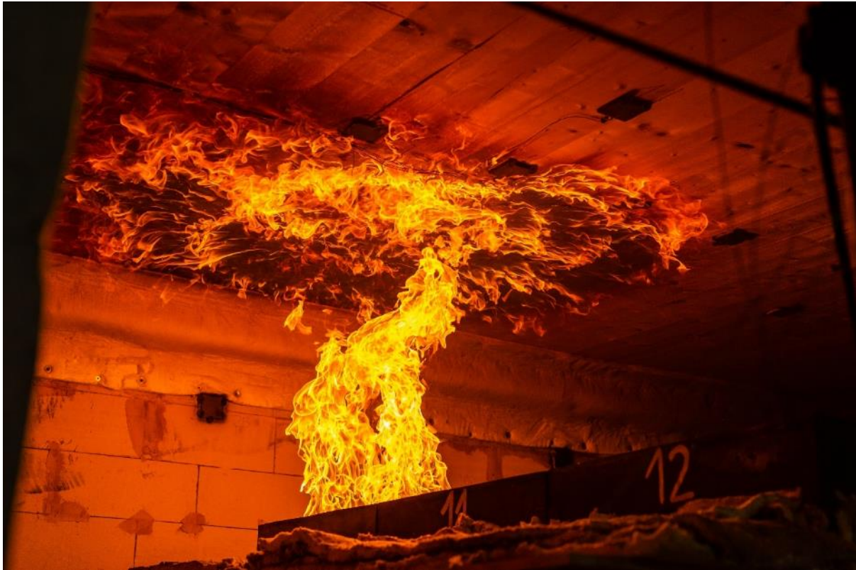
Figure 4. Flames from burner impacting ceiling in experiment 3.
