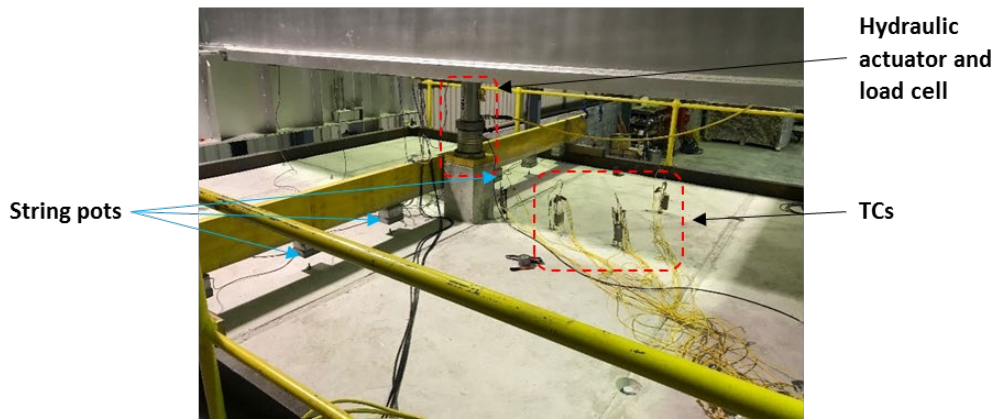
Figure 4. TCs, String pots and hydraulic actuator fixed to the specimen while it is on top of the furnace
