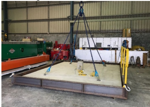
Figure 2. Slab specimen with the supporting frame before placing on the furnace
