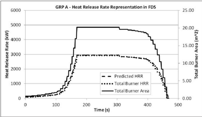
**Figure 13.** GRP A – heat release rate curve representation in FDS.
