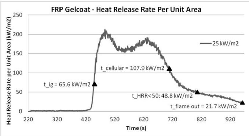
Figure 2. Representative material – 25 kW/m<sup>2</sup> cone calorimeter results.
