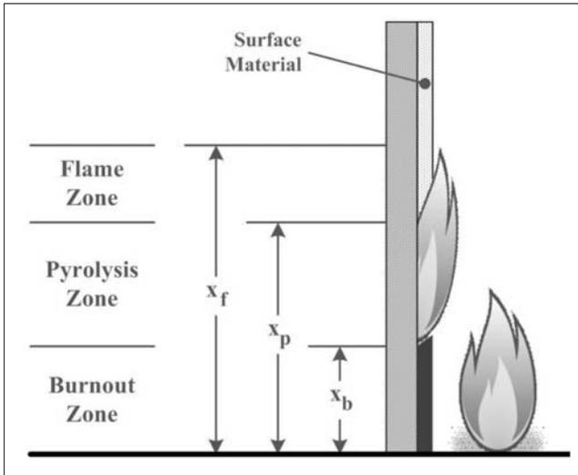
Figure 3. Upward flame spread model.
