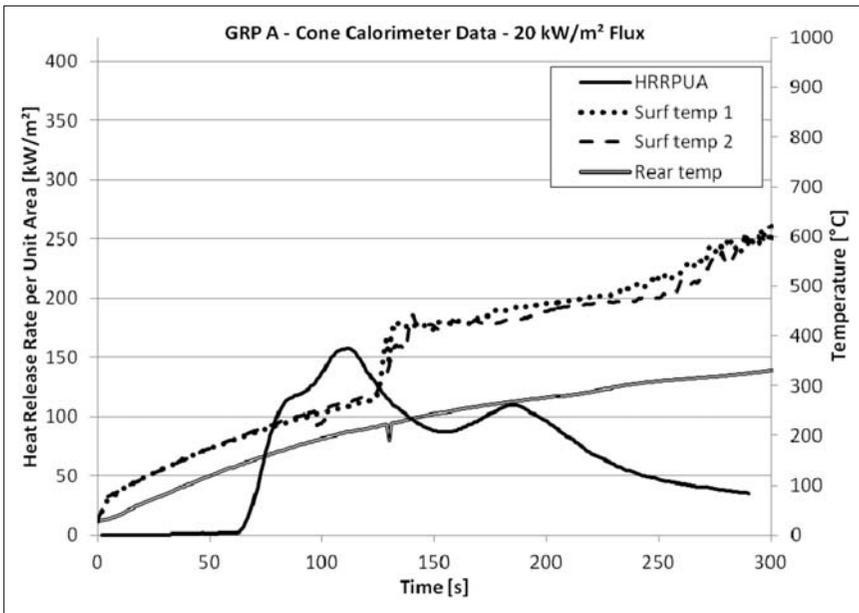
**Figure 7.** Cone calorimeter data – GRP A with 20 kW/m<sup>2</sup> flux.
