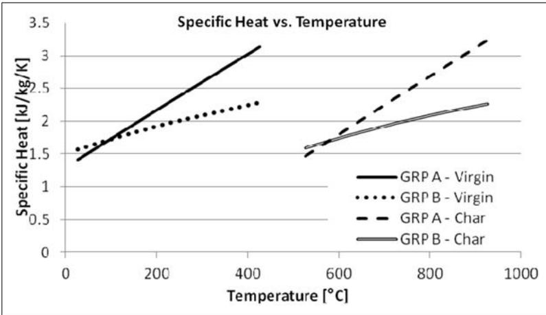
**Figure 12.** GRP specific heat temperature dependence. GRP: glass-reinforced polymer.
