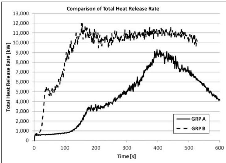
**Figure 15.** Comparison of total heat release rates from FDS.
