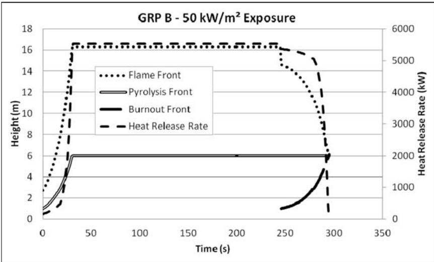
**Figure 6.** Flame spread analysis results – GRP B with 50 kW/m<sup>2</sup> exposure. GRP: glass-reinforced polymer.
