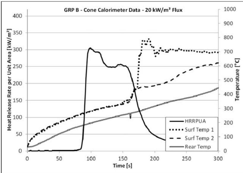
Figure 9. Cone calorimeter data – GRP B with 20 kW/m<sup>2</sup> flux.
