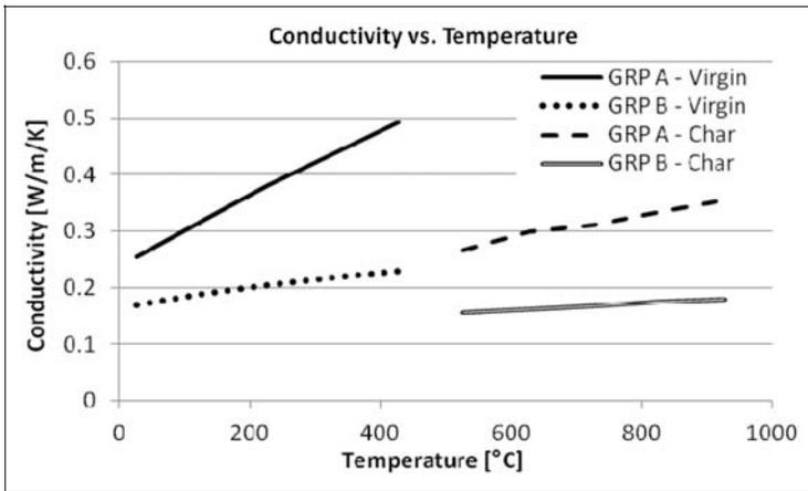
**Figure 11.** GRP conductivity temperature dependence.
