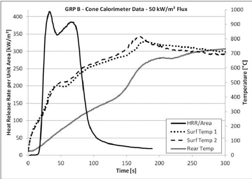
Figure 10. Cone calorimeter data – GRP B with 50 kW/m<sup>2</sup> flux. GRP: glass-reinforced polymer.
