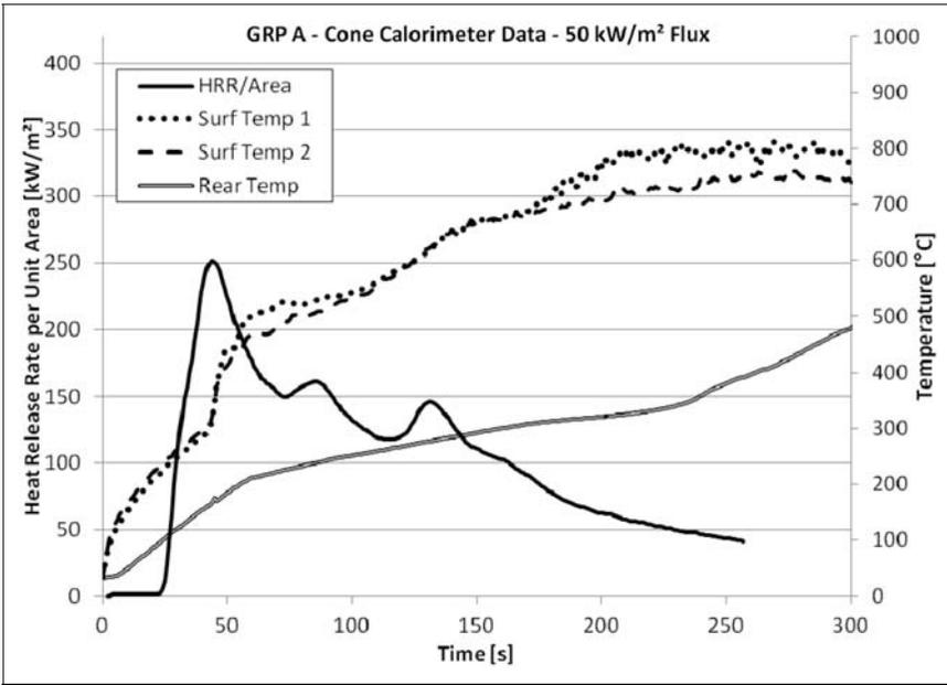
Figure 8. Cone calorimeter data – GRP A with 50 kW/m<sup>2</sup> flux.
