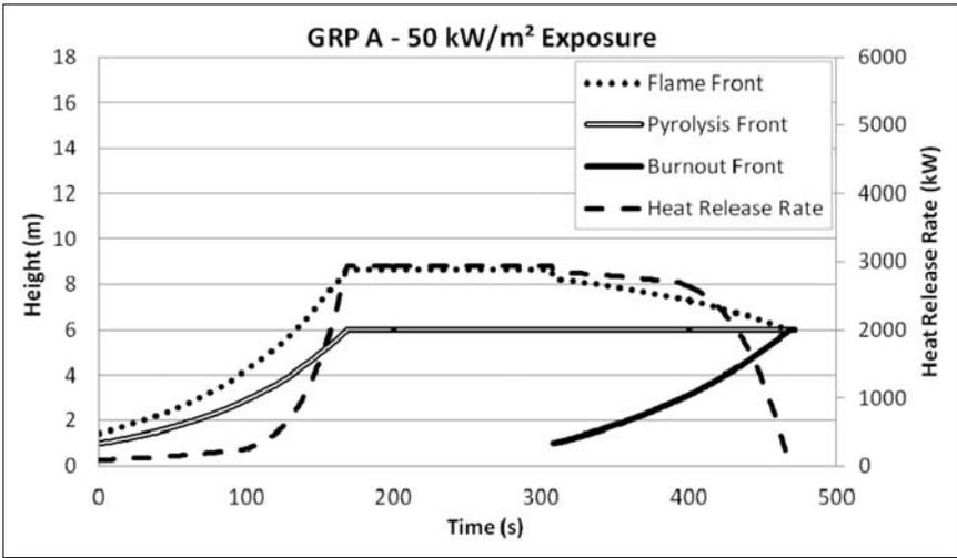
**Figure 5.** Flame spread analysis results – GRP A with 50 kW/m<sup>2</sup> exposure. GRP: glass-reinforced polymer.
