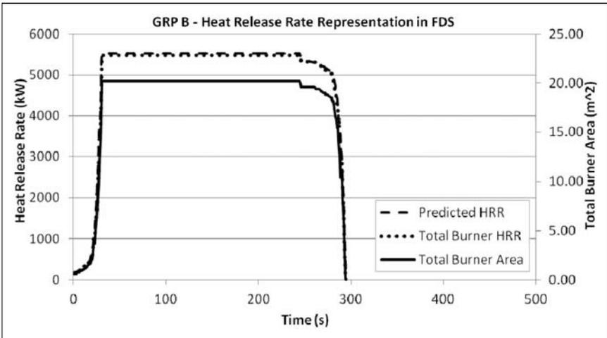
**Figure 14.** GRP B – heat release rate curve representation in FDS.
