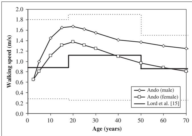
**Figure 6.** Comparison of walking speed as a function of sex and age from an adaptation of Ando et al. with mean, maximum and minimum range values (dashed lines) from Lord et al. [15].
