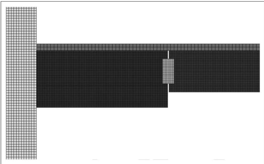
Figure 8. Assembly B thermal model (elevation view; SFRM not shown).
