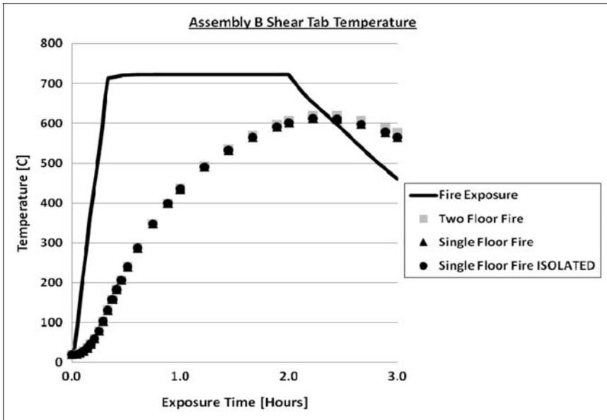
Figure 12. Assembly B shear tab temperature histories.
