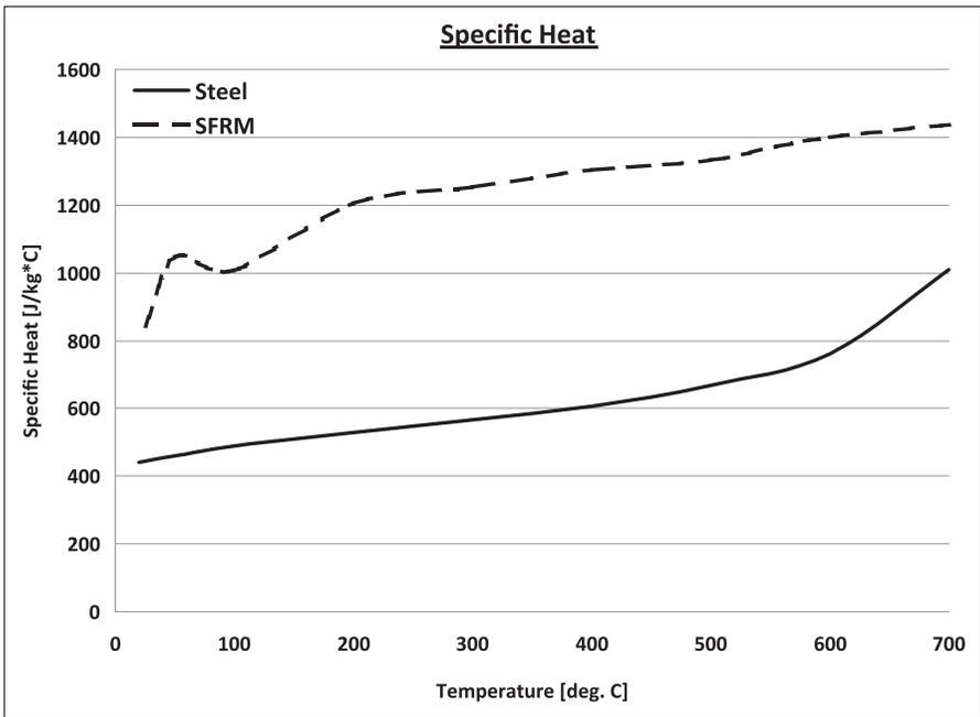
Figure 4. Temperature-dependent specific heat.
