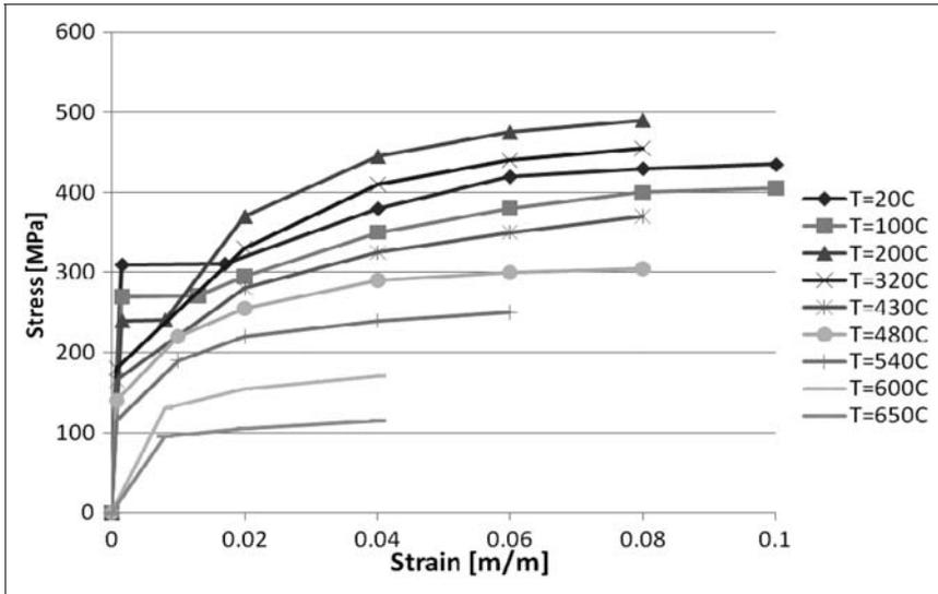
Figure 13. Temperature-dependent A36 steel strength behavior.
