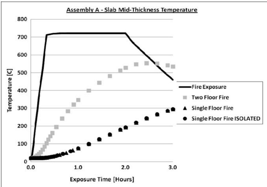
Figure 11. Assembly A slab mid-thickness temperature histories.
