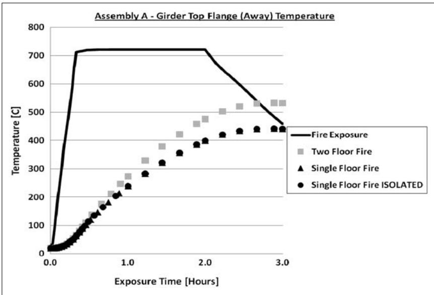
Figure 10. Assembly A girder top flange temperature histories (4 ft. away from column).
