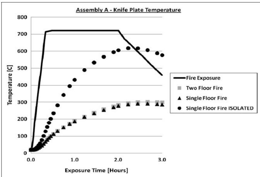
Figure 9. Assembly A knife plate temperature histories.
