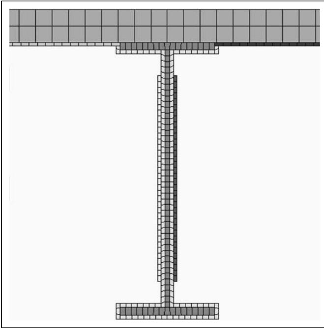
Figure 7. Assembly A thermal model (elevation view; column not shown).
