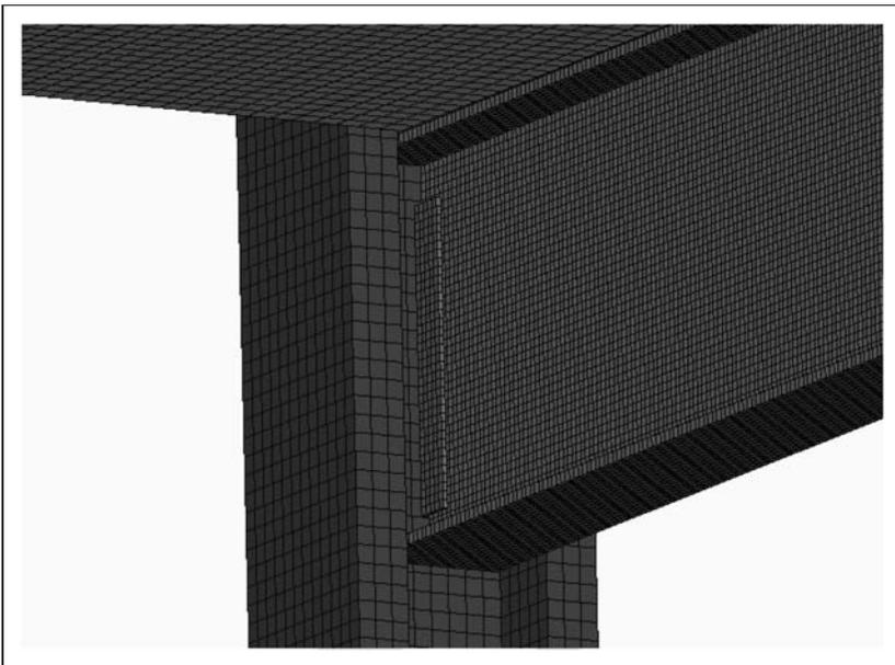
**Figure 6.** Assembly A thermal model (double knife plate connection; SFRM not shown).
