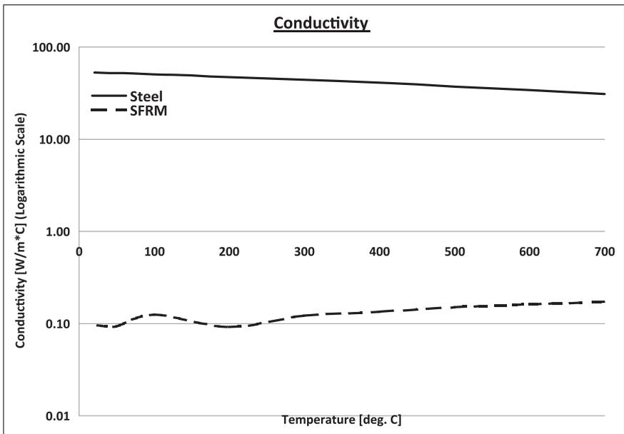
Figure 5. Temperature-dependent conductivity.
