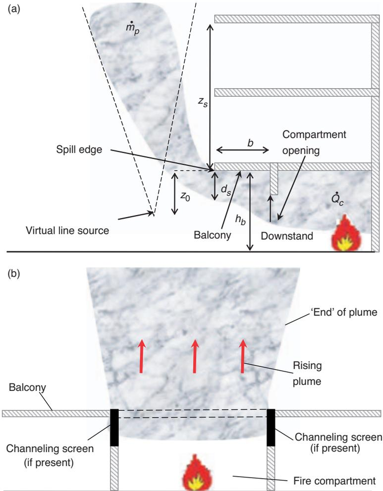
**Figure 1.** A typical 3D balcony spill plume: (a) section, (b) front view.
