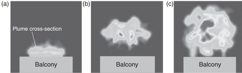
**Figure 3.** Horizontal cross-sectional area of the plume with height (Simulation STR3): (a)  $z_s = 0$  m, (b)  $z_s = 0.5$  m, (c)  $z_s = 1.0$  m.
