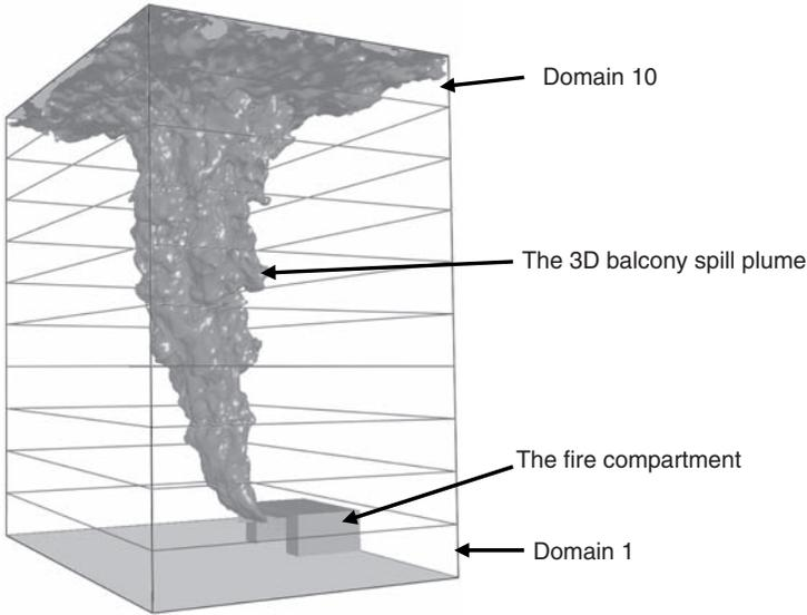
**Figure 2.** The geometry, computational domain and plume (Simulation STR3).
