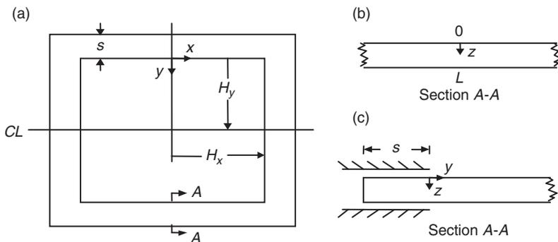
**Figure 1.** Window geometry:  $z$  is the depth,  $y$  is normal to the shaded region,  $x$  is along the shading,  $s$  is the width of the shading,  $H_y$  and  $H_x$  are the exposed pane half-lengths and  $L$  is the glass thickness. Reproduced with kind permission by the International Association for Fire Safety Science [3].
