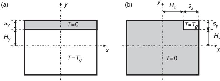
**Figure 4.** Basic geometries for multiple superposition: (a) single strip shaded, and (b) everything but corner region shaded.
