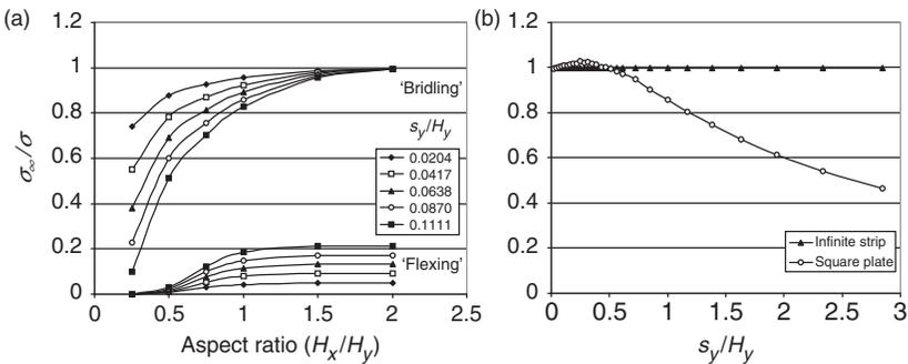
**Figure 6.** Stresses at the center of the sides normalized by the bridling stress of an infinite strip (Equation (11)): (a) for a strip of variable aspect ratio; (b) for a square window and variable shaded width ratio. The diagrams above the figures indicate the magnitudes of the superposing stresses.
