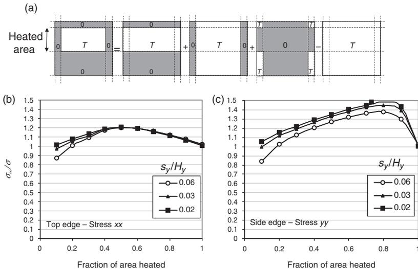
**Figure 7.** (a) Superposition of simpler configurations to represent the temperature and stress in a window with nonuniform heating, (b) top edge, and (c) side edge stresses normalized by the bridling stress in an infinite strip (Equation (11)) for variable shaded width ( $s_y/H_y$ ) and fraction of area heated.
