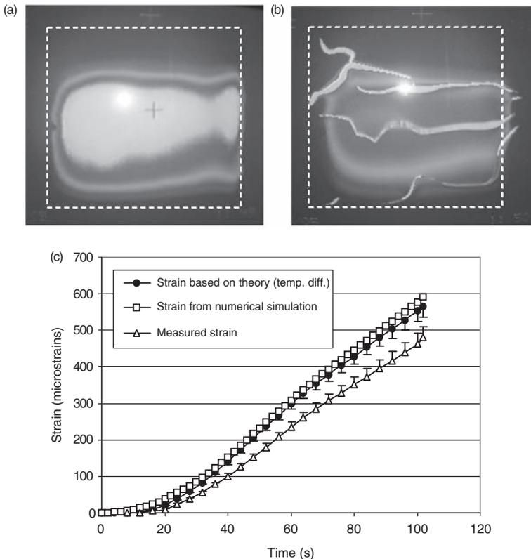
**Figure 8.** (a,b) Temperature distribution before cracking and cracking patterns on glazing, (c) Comparison of measured and calculated strains in a glazing experiment (uniform heat flux experimentally measured was used over all the window exposed area for simple calculation and numerical simulation).
