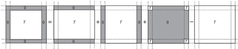
**Figure 5.** Superposition of simple configurations to represent a window with constant width of the shaded area.
