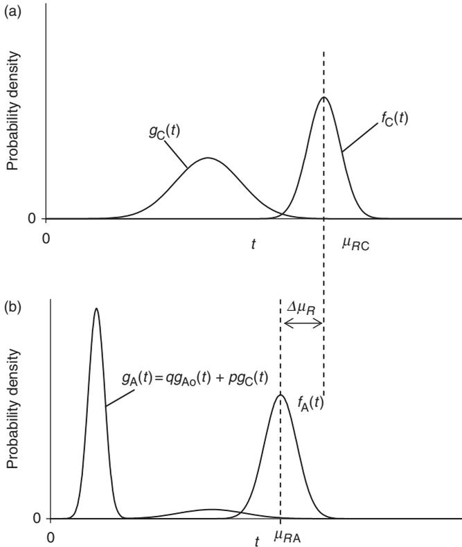
**Figure 2.** Probability density functions for fire severities and FRL in (a) a code-complying design without sprinklers and (b) an alternative solution with sprinklers.
