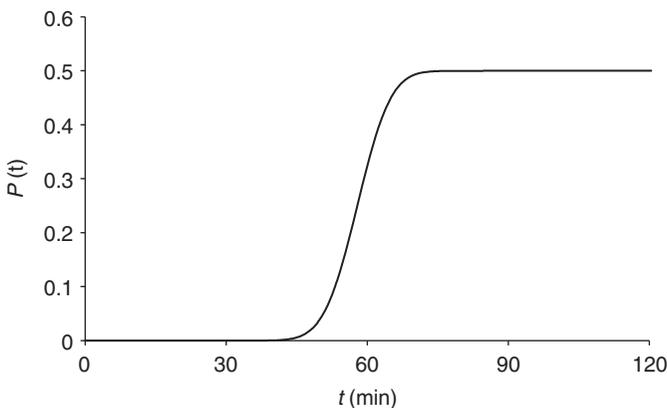
**Figure 3.** Failure probability distribution for identical  $f(t)$  and  $g(t)$  with  $\mu = 60$  min and  $\alpha = 0.1$ .
