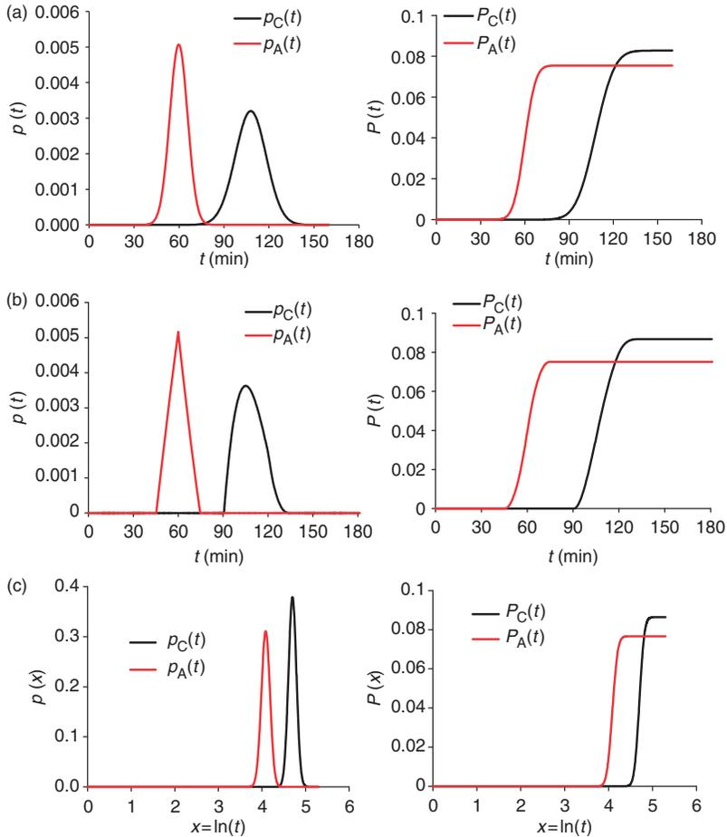
**Figure 5.** Fire resistance failure probability density and probability functions for three types of source distributions. ( $q = 0.92$ ,  $\mu_{RA} = 60$  min): (a) normal distribution, (b) triangle distribution, (c) lognormal distribution. (The color version of this figure is available online.)
