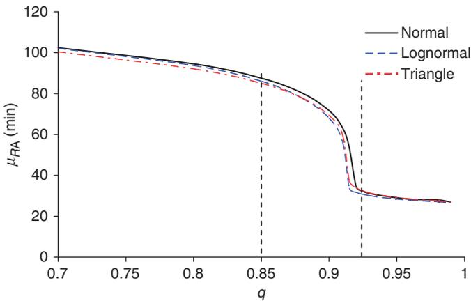
**Figure 4.** Variation of the required FRL with sprinkler reliability. (The color version of this figure is available online.)
