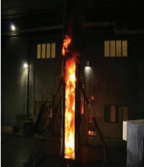
**Figure 4.** Fire propagation over material in 4.9-m high parallel panel test. (The color version of this figure is available online.)
