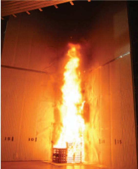
**Figure 2.** The 50-ft corner test with polyisocyanurate foam panels covered with a steel facing. (The color version of this figure is available online.)
