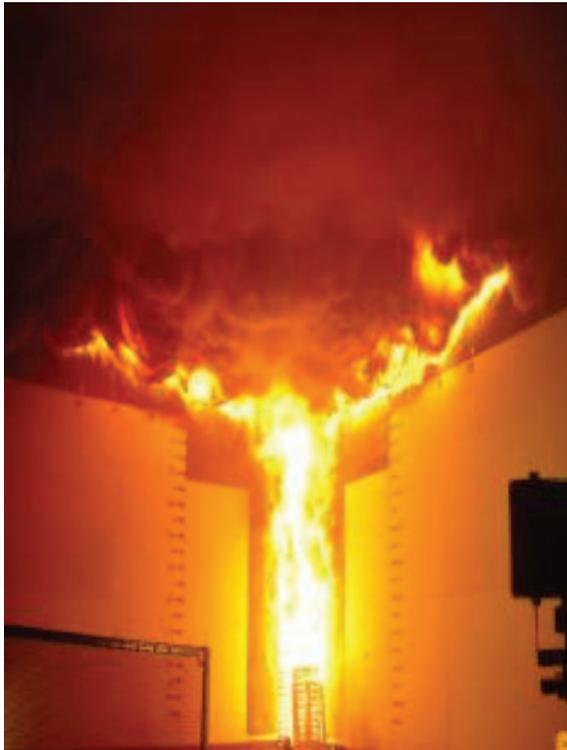
**Figure 1.** The 25-ft corner test with PVC panels. (The color version of this figure is available online.)
