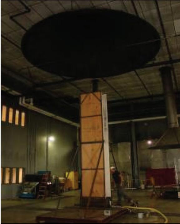
**Figure 3.** New 4.9-m high parallel panel test apparatus under 5-MW FPC. (The color version of this figure is available online.)
