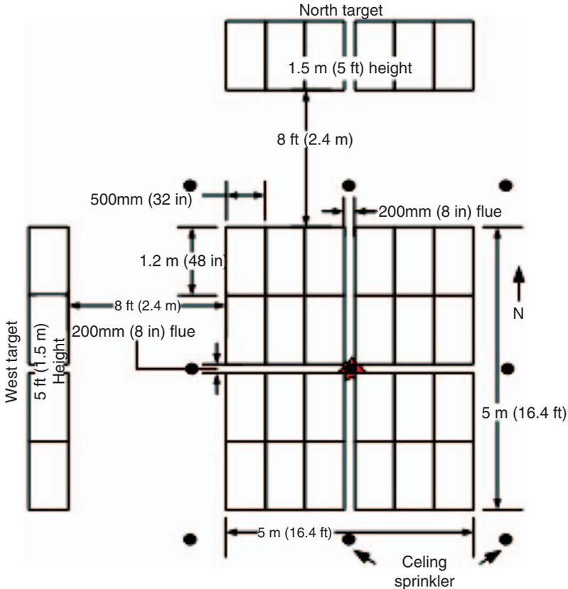
**Figure 2.** Plan view of test arrangement with location of the nine (9) ignition zone sprinklers. (The color version of this figure is available online.)
