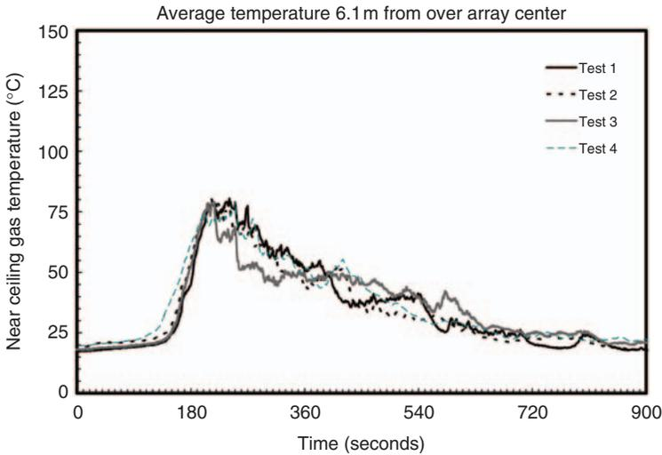
**Figure 11.** Average near-ceiling gas temperature at 6.1 m radius. (The color version of this figure is available online.)
