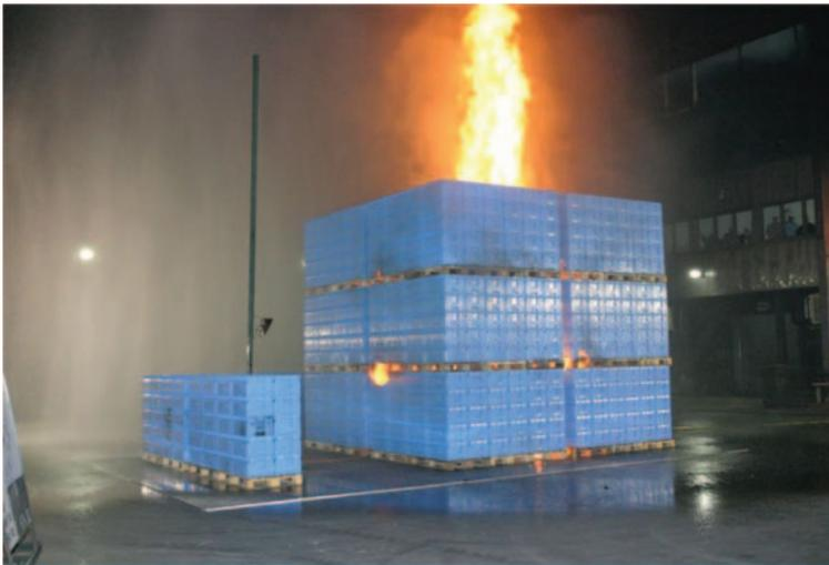
**Figure 13.** *Flames at transverse and longitudinal flue openings (Test 4). (The color version of this figure is available online.)*
