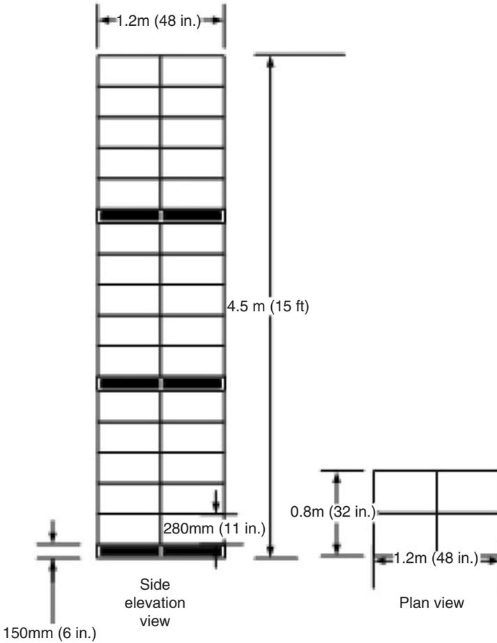
**Figure 3.** Single stack configuration of KLT plastic totes.
