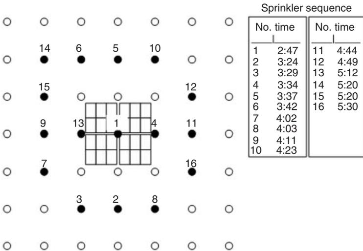
Figure 6. Sprinkler actuation sequence – Test 3 – plain water system (filled symbols represent actuated sprinklers).
