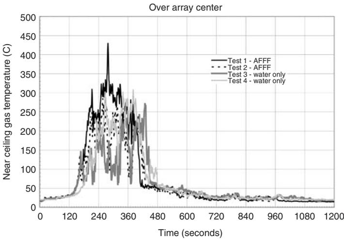
Figure 8. Near-ceiling gas temperature over ignition.
