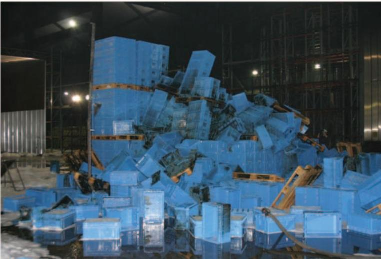
**Figure 14.** Test 1 – post test (view from north-east corner). Test duration: 22 minutes. (The color version of this figure is available online.)
