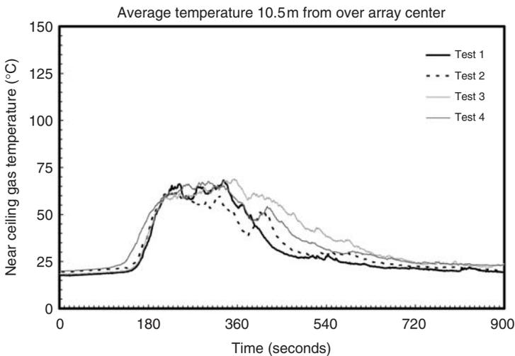
**Figure 12.** Average near-ceiling gas temperature at 10.5 m radius.
