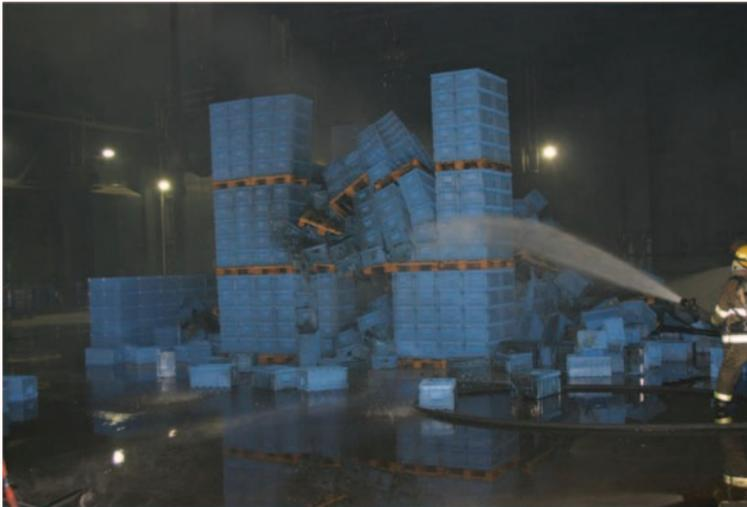
**Figure 16.** Test 3 – Post test (view from south-east corner). Test duration: 25 minutes. (The color version of this figure is available online.)
