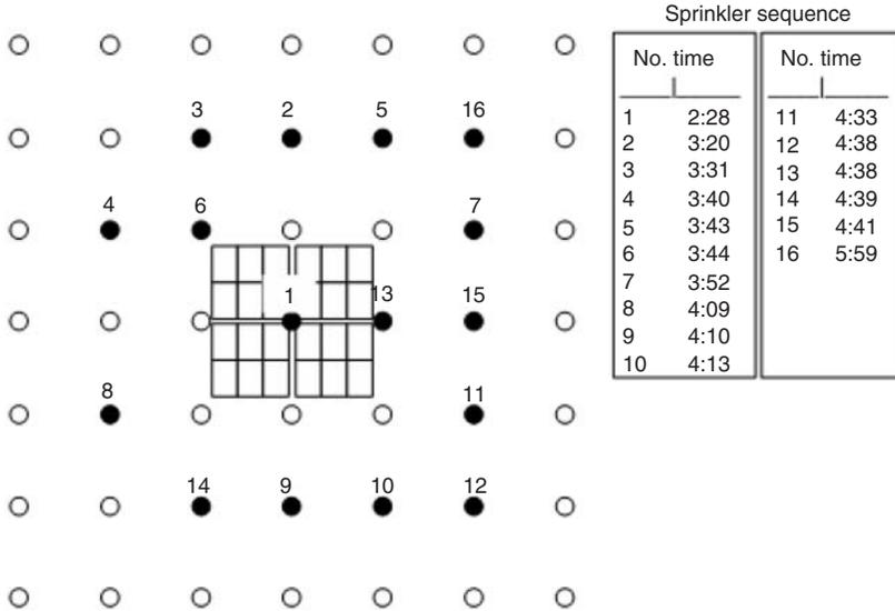
Figure 7. Sprinkler actuation sequence – Test 4 – plain water system (repeat of Test 3).
