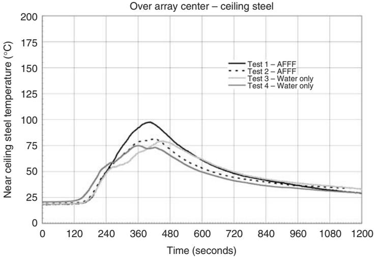
Figure 9. Ceiling steel temperature over ignition.
