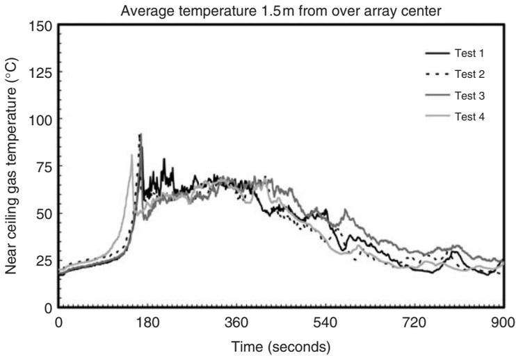
Figure 10. Average near-ceiling gas temperature at 1.5m radius.
