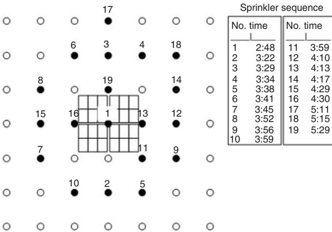
**Figure 4.** Sprinkler actuation sequence – Test 1 – AFFF system (filled symbols represent actuated sprinklers).
