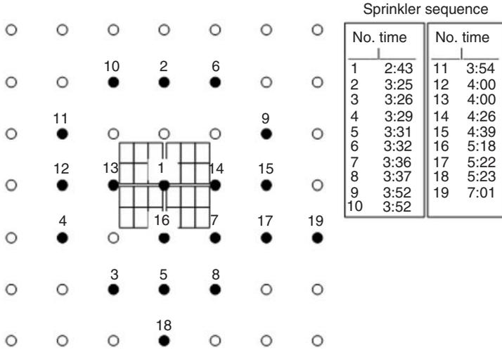
Figure 5. Sprinkler actuation sequence – Test 2 – AFFF system (repeat of Test 1).
