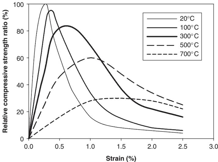
**Figure 1.** Stress–strain relationships for concrete at elevated temperature (simplified and redrawn according to EC2 [15]).
