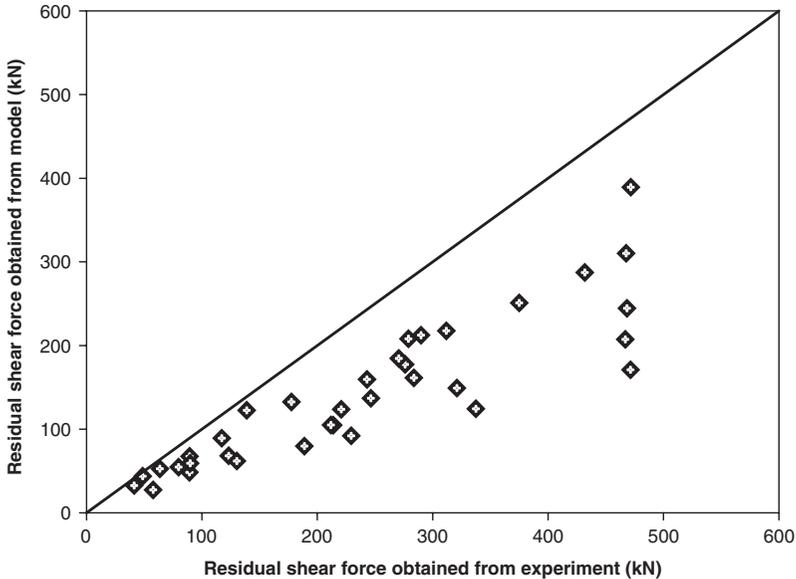
**Figure 13. Comparison of residual shear forces obtained from experimental and modeling results.**
