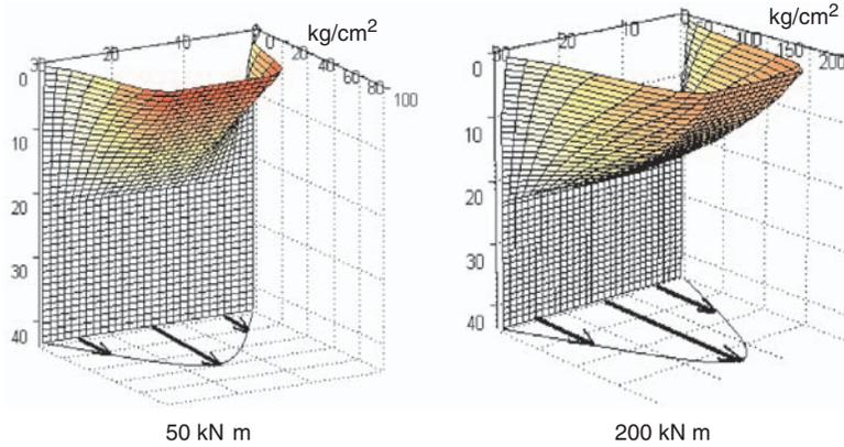
**Figure 3.** Thermal stress distribution under different torque loads after 2.5 hours of fire exposure.
