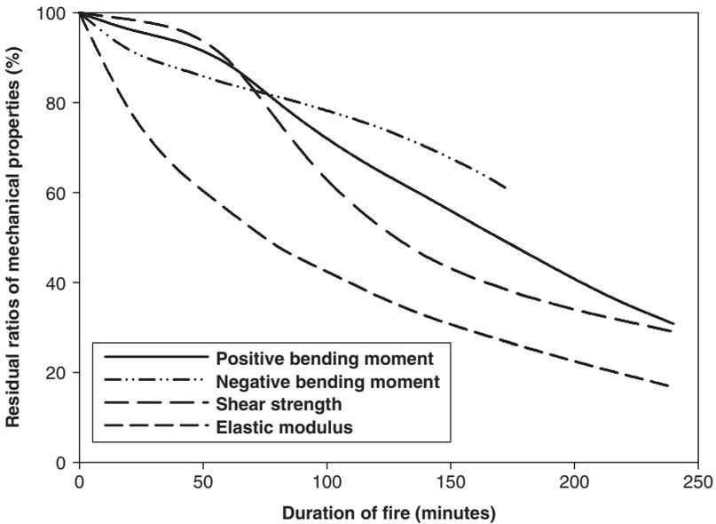
Figure 17. Residual ratios of bending moment, shear force and elastic modulus as a function of duration of fire exposure.
