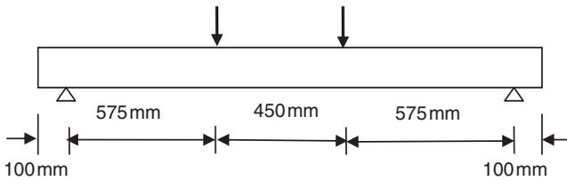
Figure 10. Fire flexural test conditions.
