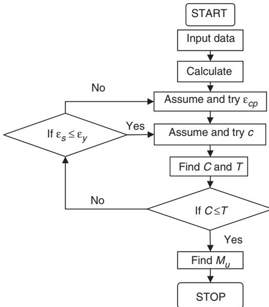
**Figure 2.** Flowchart for calculated residual flexural capacity of RC beam exposed to fire.
