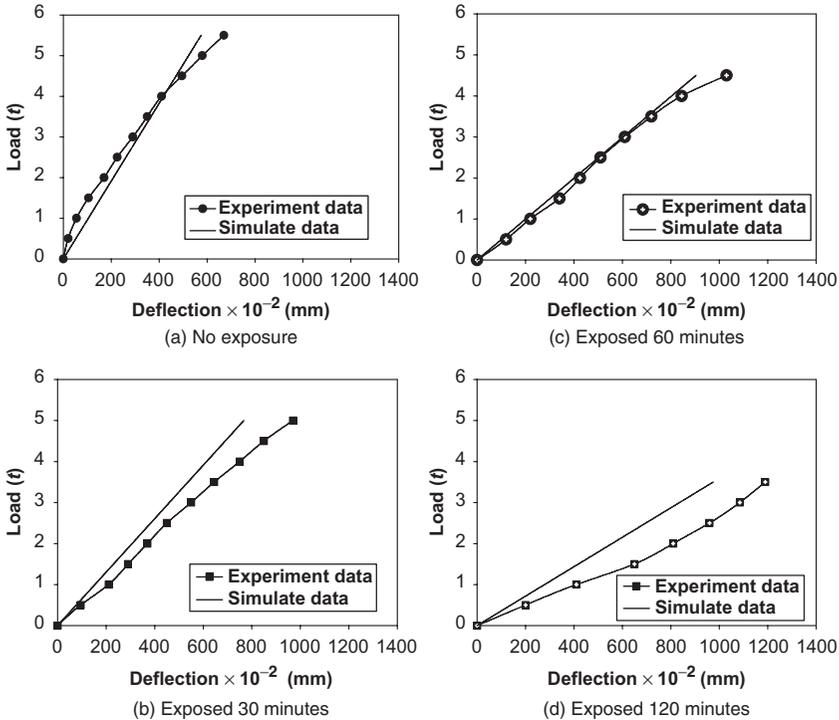
**Figure 14.** Comparison between experimental and simulated data with various durations of fire exposure.
