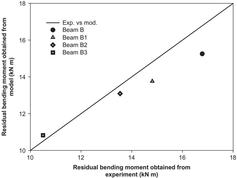
Figure 11. Comparison of residual bending moments obtained from experimental and modeling results.
