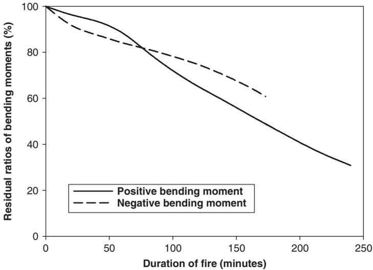
**Figure 15.** Residual ratios of positive and negative bending moments as a function of duration of fire exposure.
