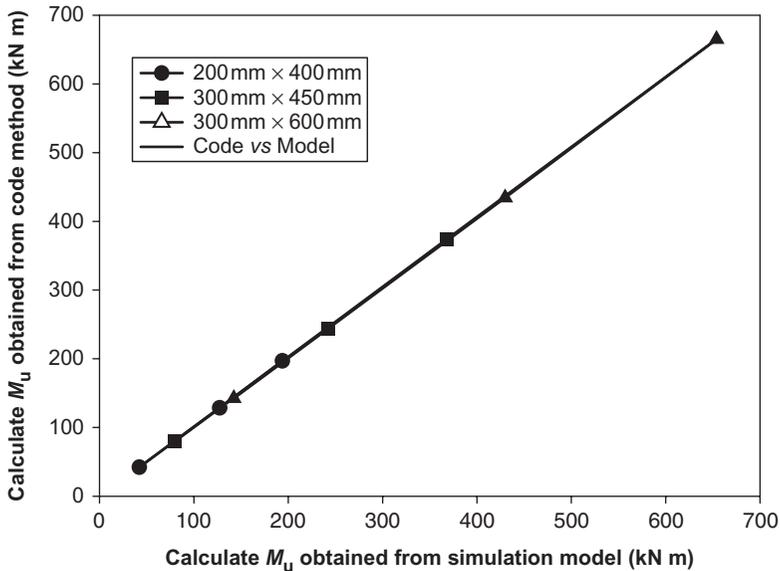
**Figure 8.** Comparison of ultimate bending moment ( $M_u$ ) obtained from the ACI Code method and simulated results for various dimensions of beams and steel ratios.
