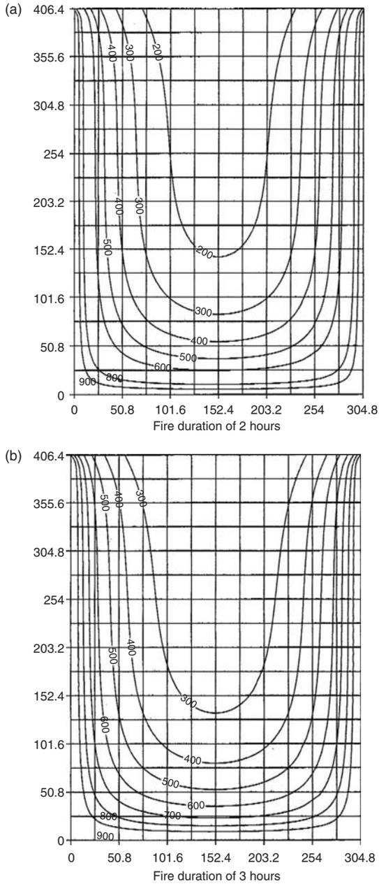
Figure 7. Comparison of isothermal contours in concrete beams during fire exposure.
