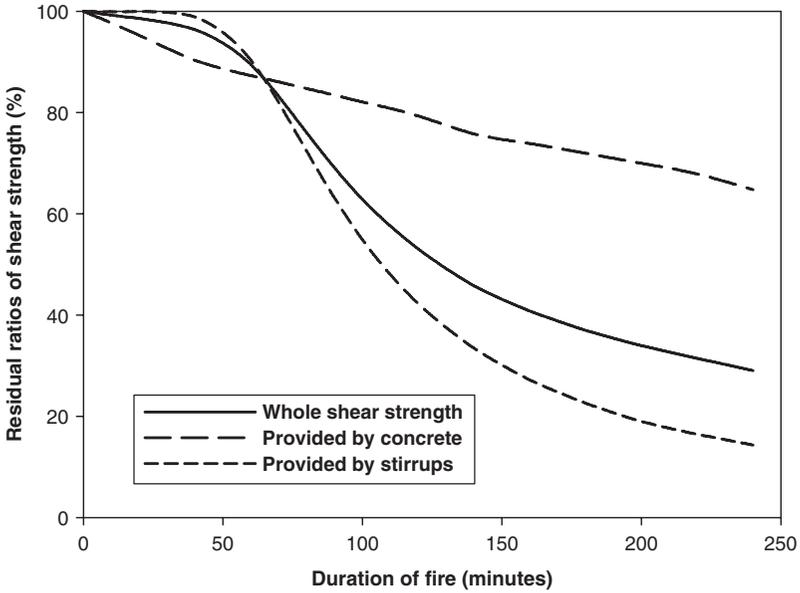
Figure 16. Residual ratios of shear force as a function of duration of fire exposure.
