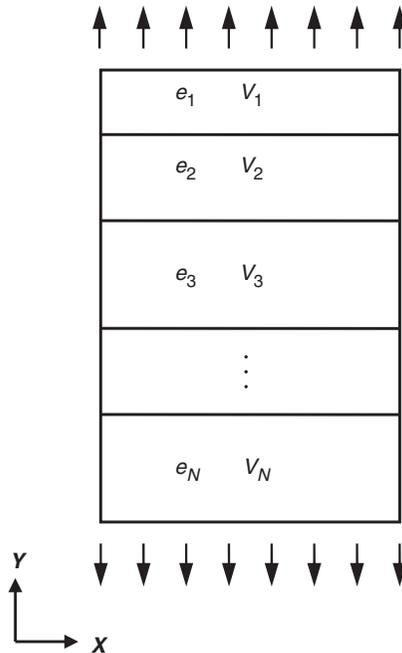
**Figure 6.** Parallel strip (with different horizontal elastic moduli).
