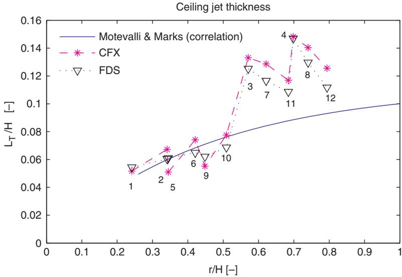
**Figure 12.** Comparison of thickness of ceiling jet based on temperature for the 12 different sprinkler positions using correlation of Motevalli and Marks, CFX and FDS,  $t = 140$  seconds (The color version of this figure is available online).
