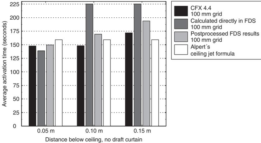
**Figure 13.** Average activation time of sprinklers at three different positions calculated with CFX, FDS, and Alpert's ceiling jet formula.
