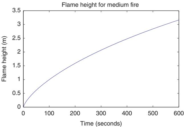
**Figure 3.** Flame height calculated using Heskestad's formula (The color version of this figure is available online).
