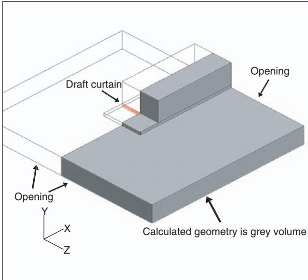
**Figure 4.** Modeled geometry in CFX is the gray area (The color version of this figure is available online).
