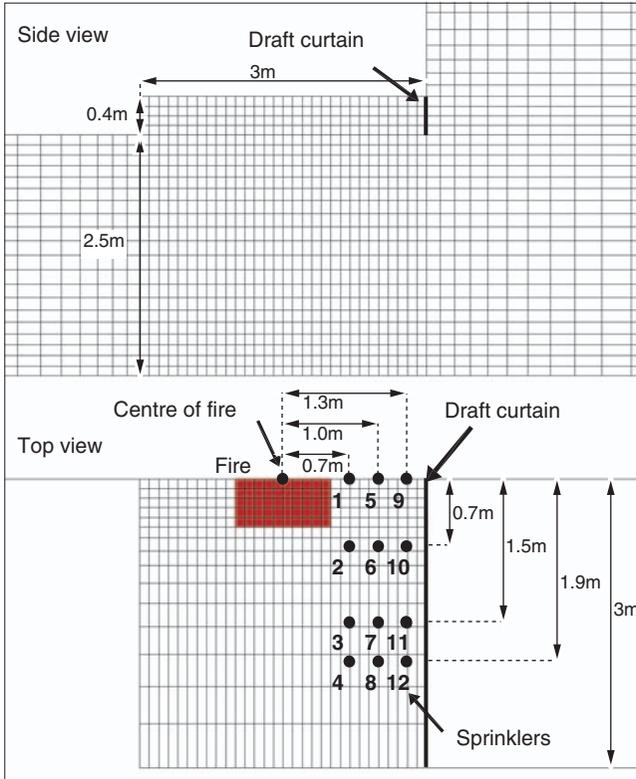
**Figure 5.** Area around raised ceiling with sprinkler positions (symmetry plane through the middle for the CFX simulation) (The color version of this figure is available online).
