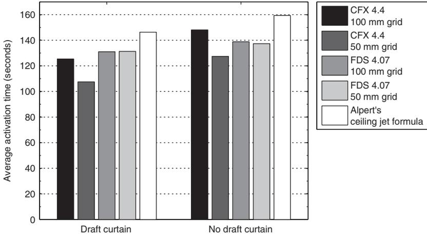
**Figure 14.** Average activation time of sprinklers placed in the middle of the first cell in CFX and FDS, and compared to Alpert’s ceiling jet formula. Values are taken at middle of first node.
