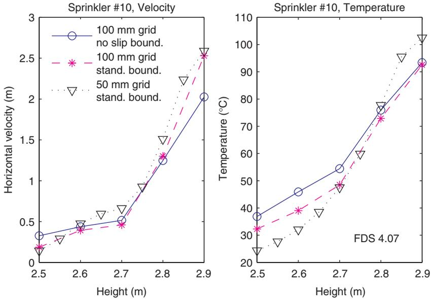
**Figure 10.** Velocity and temperature profile in the ceiling jet for three different FDS simulations with no draft curtain at sprinkler position 10 ( $r=1.48$  m),  $t=140$  seconds (The color version of this figure is available online).
