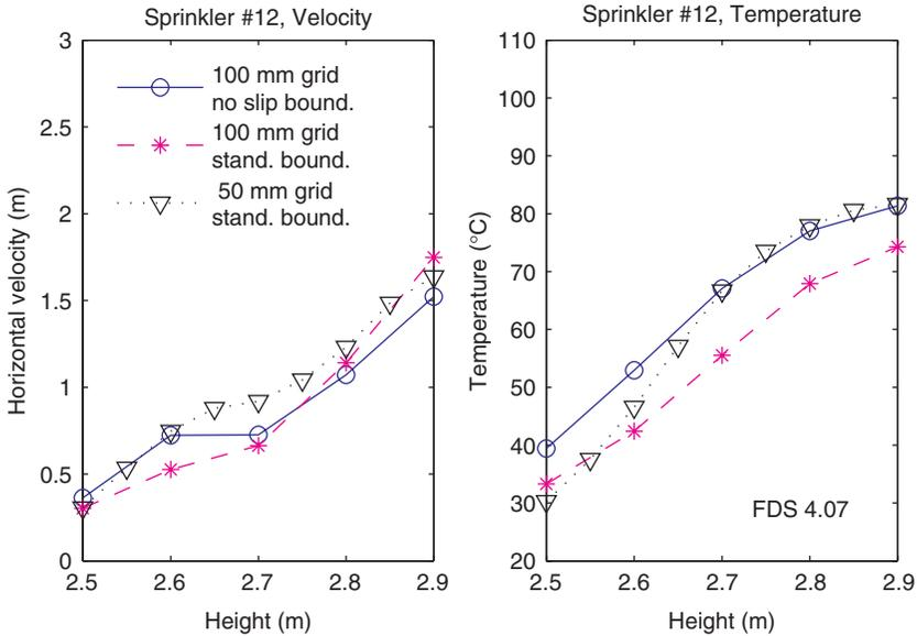
**Figure 11.** Velocity and temperature profiles in the ceiling jet for three different FDS simulations with no draft curtain at sprinkler position 12 ( $r=2.3\text{ m}$ ),  $t=140\text{ seconds}$  (The color version of this figure is available online).
