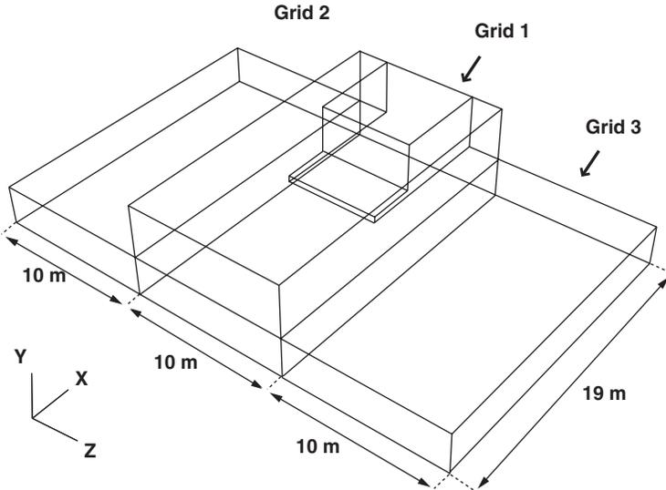
Figure 7. The geometry in FDS is modeled with three different grids and blocked out cells.
