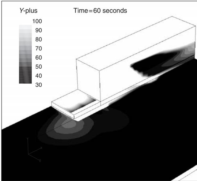
Figure 6. Y-plus value for a CFX 4.4 simulation with fine grid and draft curtain,  $t=60$  seconds.
