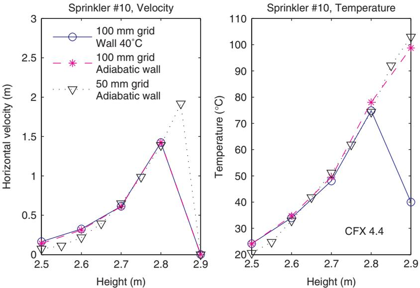
**Figure 8. Velocity and temperature profile in the ceiling jet for three different CFX simulations with no draft curtain at sprinkler position 10 ( $r = 1.48$  m),  $t = 140$  seconds (The color version of this figure is available online).**
