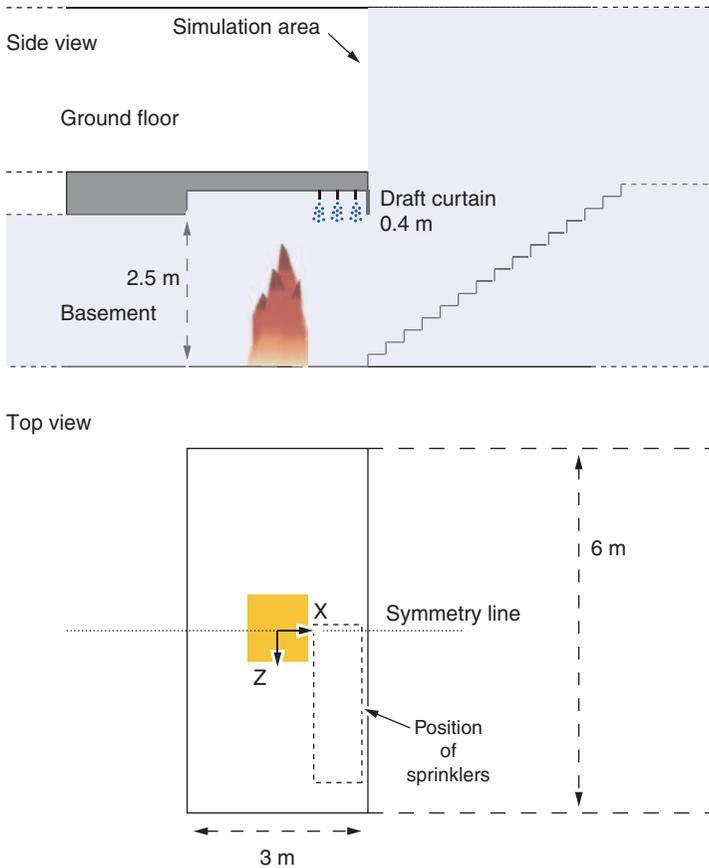
**Figure 1.** Geometry of raised ceiling and draft curtain (The color version of this figure is available online).
