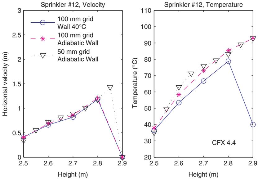
**Figure 9.** Velocity and temperature profile in the ceiling jet for three different CFX simulations with no draft curtain at sprinkler position 12 ( $r=2.3$  m),  $t=140$  seconds (The color version of this figure is available online).
