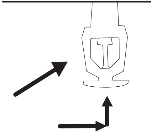
**Figure 2.** Deflector plate shields the sprinkler bulb from vertical velocities.
