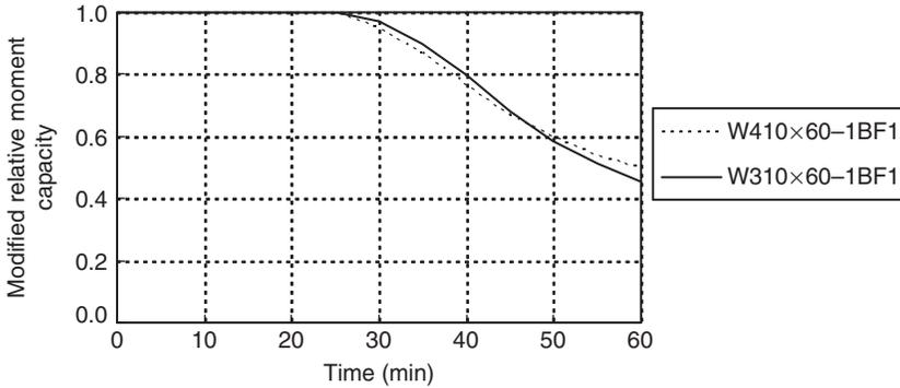
**Figure 16.** Modified relative cross-section moment capacities for 1-hour rating W410 × 60 and W310 × 60 beams with protection loss on the bottom flange.
