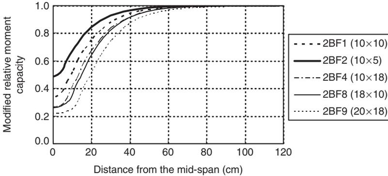
**Figure 18.** Modified relative cross-section moment capacities after 1 hour of standard fire exposure for 1-hour rating  $W410 \times 74$  beams with symmetric bottom flange protection loss.
