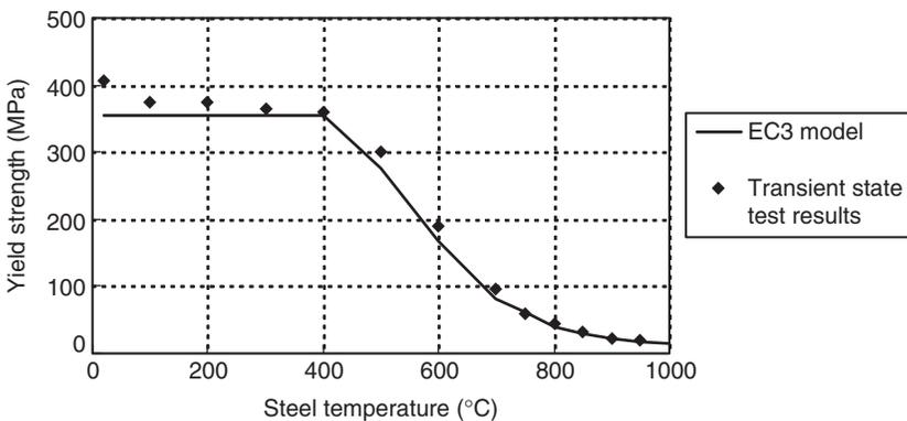
**Figure 1.** Yield strength of structural steel S355 at elevated temperatures (adopted from Outinen et al. [7]).
