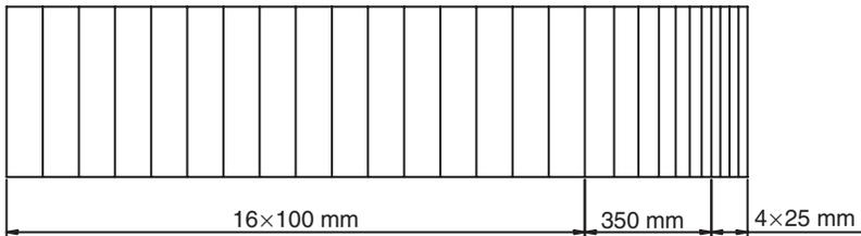
Figure 5. Longitudinal mesh.
