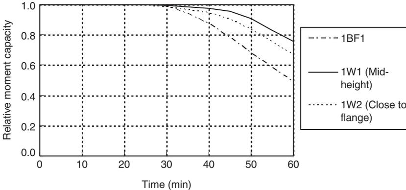
**Figure 12.** Relative cross-section moment capacities for 1-hour rating W410 × 74 beams with protection loss on the bottom flange or on the web.
