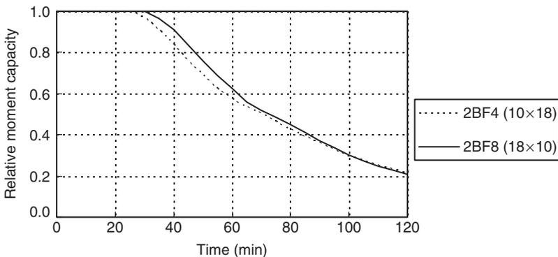
**Figure 10.** Relative cross-section moment capacities for  $W410 \times 74$  beams 2BF4 and 2BF8.
