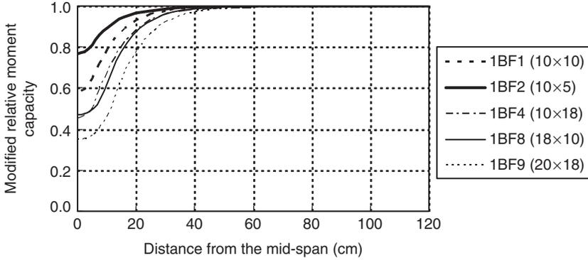
**Figure 17.** Modified relative cross-section moment capacities after 1 hour of standard fire exposure for 1-hour rating  $W410 \times 74$  beams with symmetric bottom flange protection loss.
