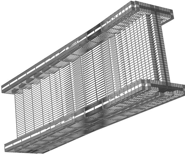
**Figure 3.** Finite element heat transfer model of a beam with protection loss on the bottom flange.
