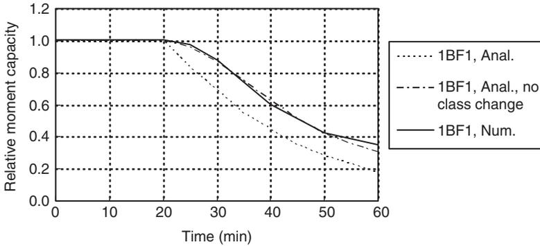
**Figure 19.** Relative cross-section moment capacities for 1-hour rating  $W310 \times 39$  beams with symmetric bottom flange protection loss.
