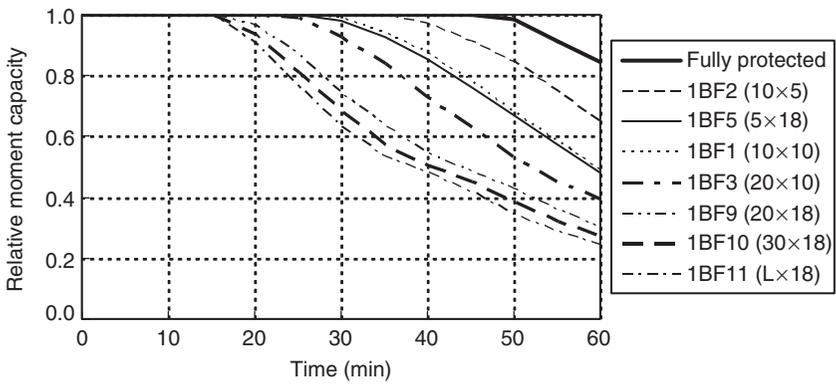
**Figure 8.** Relative cross-section moment capacities for 1-hour rating  $W410 \times 74$  beams with symmetric bottom flange protection loss.
