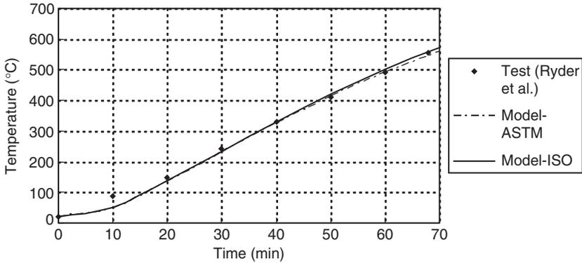
Figure 6. Average temperature of a W10 × 49 steel column with 19 mm of protection.
