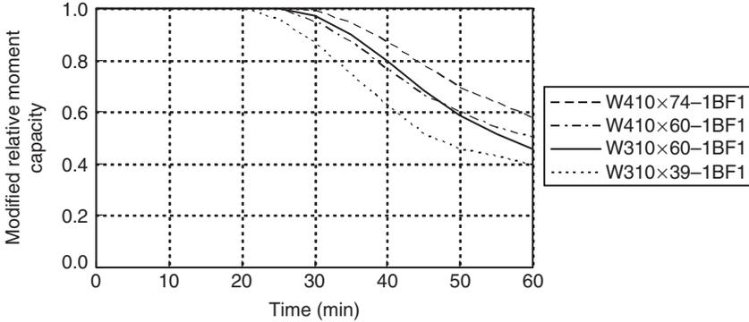
**Figure 15.** Modified relative cross-section moment capacities for 1-hour rating W410 × 74, W410 × 60, W310 × 60, and W310 × 39 beams with protection loss on the bottom flange.
