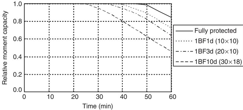
**Figure 14.** Relative cross-section moment capacities for 1-hour rating  $W410 \times 74$  beams with full protection and with an 87.5% penetrated bottom flange protection loss.
