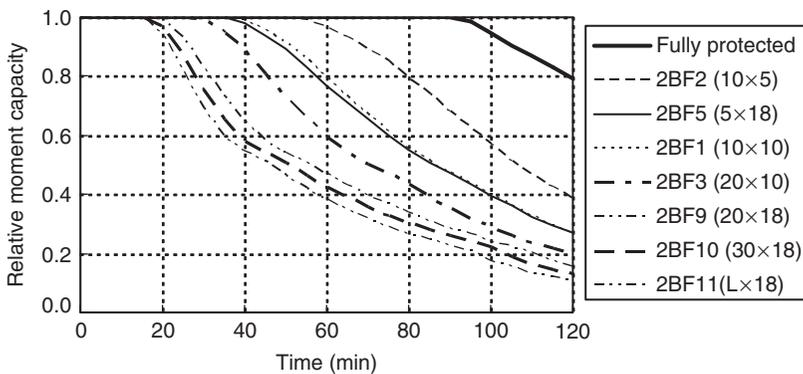
**Figure 9.** Relative cross-section moment capacities for 2-hour rating  $W410 \times 74$  beams with symmetric bottom flange protection loss.
