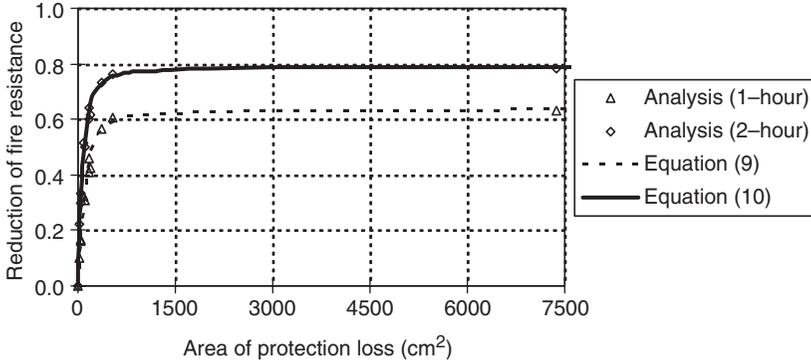
**Figure 11.** Fire resistance reductions of 1- and 2-hour rating W410 × 74 beams with the bottom flange protection loss.
