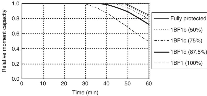
**Figure 13.** Relative cross-section moment capacities for 1-h rating W410 × 74 beams with various depths of bottom flange protection loss.
