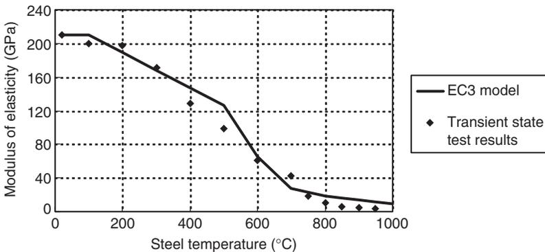
**Figure 2.** Modulus of elasticity of structural steel at elevated temperatures (adopted from Outinen et al. [7]).
