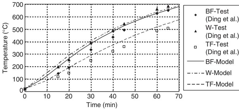
Figure 7. Temperatures of the bottom flange (BF), top flange (TF), and web (W) for an H-400 × 200 × 8 × 13 steel beam with 11.3 mm of protection.
