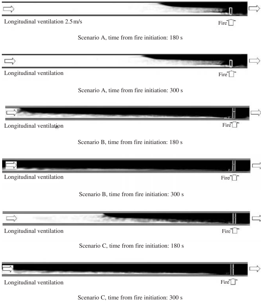
Figure 4. Side view of smoke back-layering for scenarios A, B, and C (total length shown: 130 m with 120 m upwind and 10 m downwind of the fire). Scenario A, time from fire initiation: 180 s.
