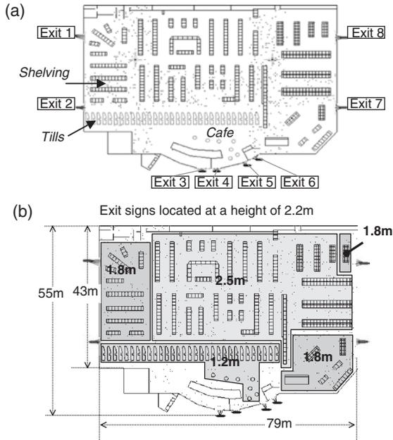
**Figure 11.** The supermarket layout as represented within the buildingEXODUS model: (a) showing location of exits and shelving and (b) indicating the height of the various internal features of the supermarket.
