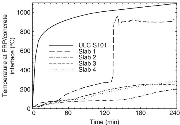
**Figure 2.** Temperature as function of time at the FRP–concrete bondline for insulated FRP-strengthened reinforced concrete slabs [21,22].
