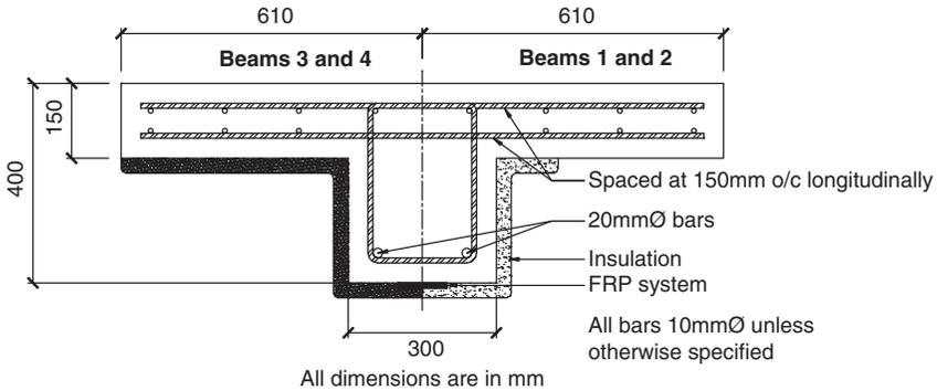
**Figure 5.** Overall dimensions, reinforcement details, FRP-strengthening scheme, and insulation scheme for beam-slab assemblies [27].
