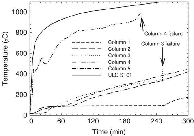
**Figure 3.** Temperature as function of time at the FRP–concrete bondline for insulated FRP-strengthened (confined) reinforced concrete columns [17,23,24].
