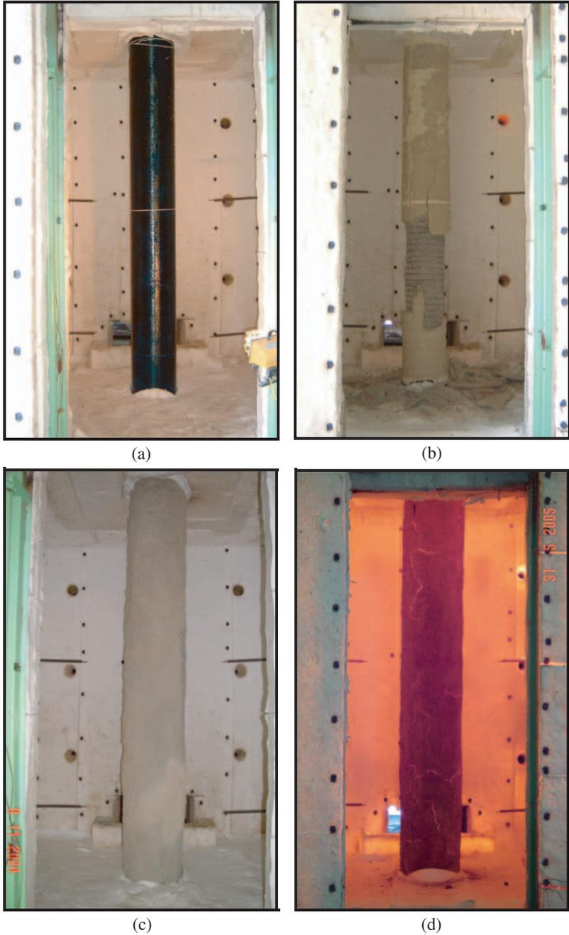
**Figure 4.** Columns 4 (a, b) and 5 (c, d) immediately before fire testing and immediately after failure during fire testing, respectively. (The color version of this figure is available on-line.)
