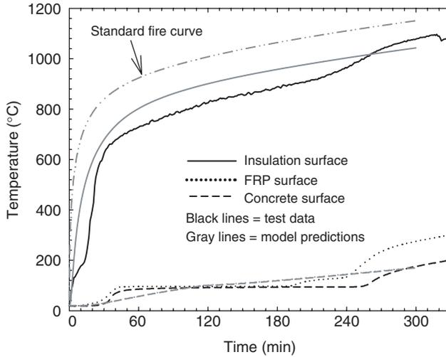
**Figure 7.** Predicted and recorded temperatures at various key locations in column 1 during fire testing [23].
