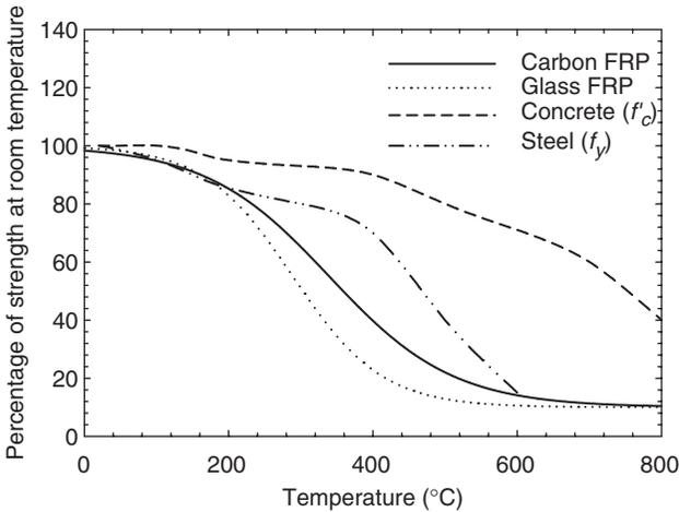
**Figure 1.** Approximate variation in strength of FRP [17] and concrete and steel [8] with increasing temperature.
