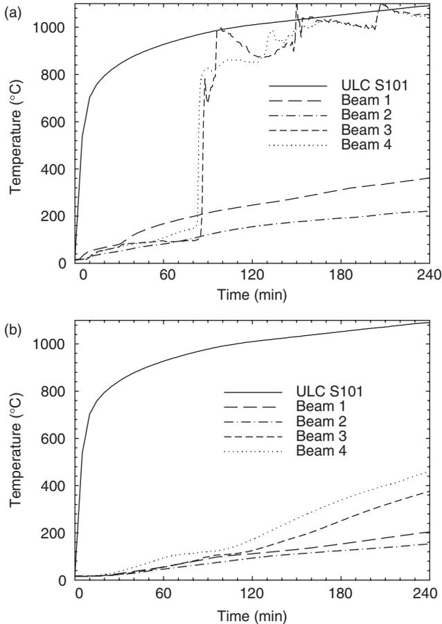
**Figure 6.** Recorded temperature as a function of time at (a) the FRP-concrete bondline and (b) the level of the internal tensile steel reinforcement for insulated FRP-strengthened reinforced concrete beam-slab assemblies [26,27].
