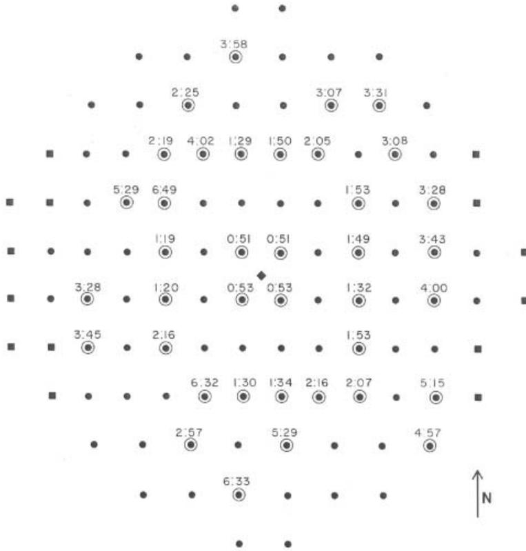
**Figure 15.** Sprinkler operating sequence of Test 10. ● – timed sprinklers; ■ – nontimed sprinklers; ⊙ – operated sprinklers; ◆ – fire center.
