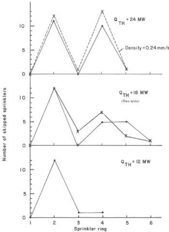
Figure 9. Skipping patterns for water discharge density 0.2 mm/s except where indicated.
