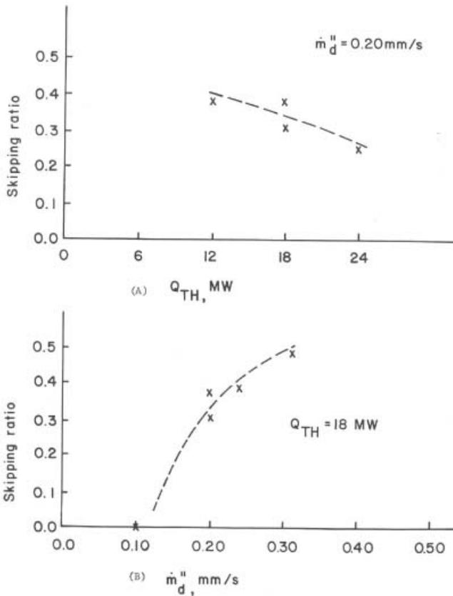
**Figure 14.** Skipping ratio as a function of (A) heat release rate and (B) water discharge density.
