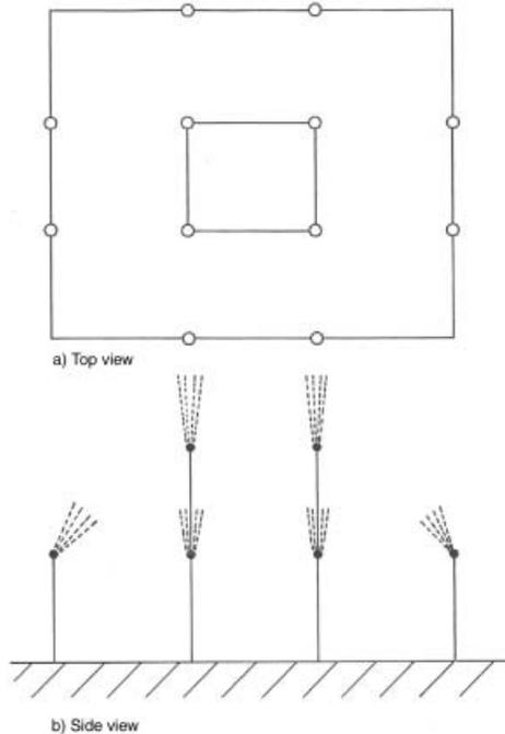
**Figure 5.** Heptane spray nozzle arrangement for the spray fire facility.
