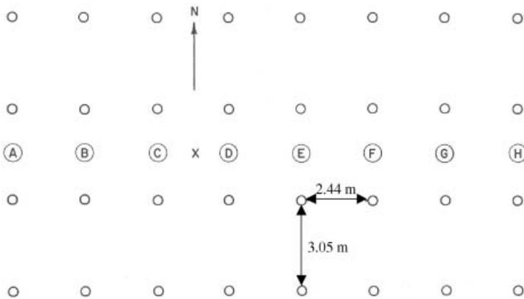
**Figure 6.** Components and locations of instrument packages. A and H – aspirated TC, DISC, and bare-bead TC; B and E–G psychrometric probe, DISC and bare-bead TC; C – none; D – aspirated and bare-bead TC; × – fire center.
