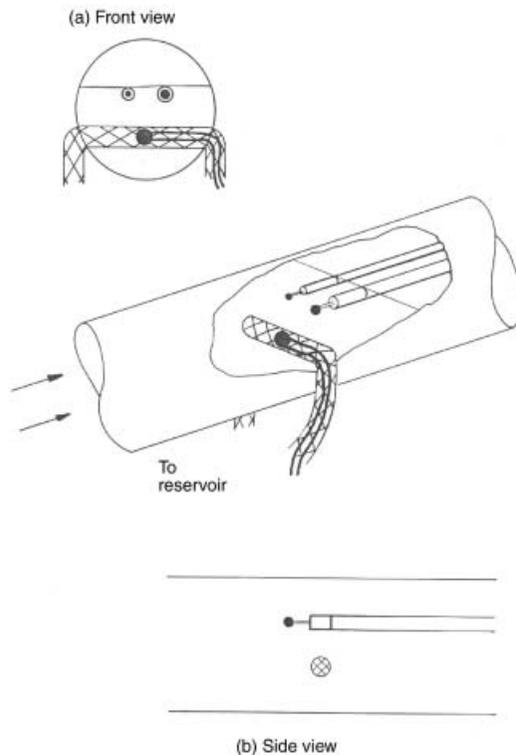
**Figure 4.** Fire environment psychrometric probe.
