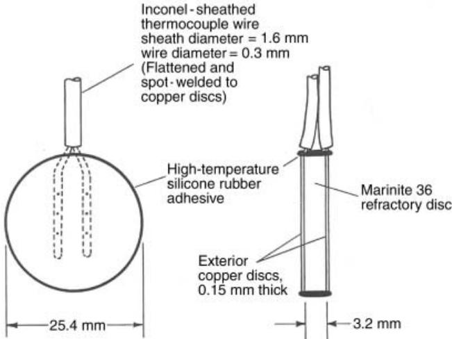
**Figure 3.** Droplet impingement, spray cooling meter (DISC).
