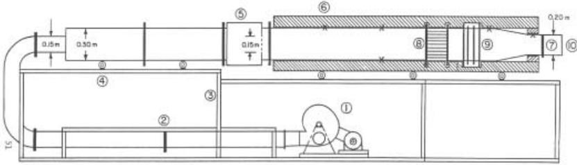
**Figure 2.** Schematic of the heated wind tunnel. The numbered components are (1) fan; (2) orifice plate; (3) support frame; (4) roller; (6) burner chamber; (7) feedback TC; (8) flow straightener tube; (9) flow smoothing screens; (10) test area; × – thermocouples.
