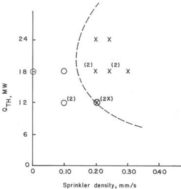
**Figure 7.** The occurrence of skipping as a function of fire intensity and water discharge density. The dashed line stands for a possible boundary between skipping and nonskipping behavior.  $\times$  – skipping;  $o$  – non-skipping.
