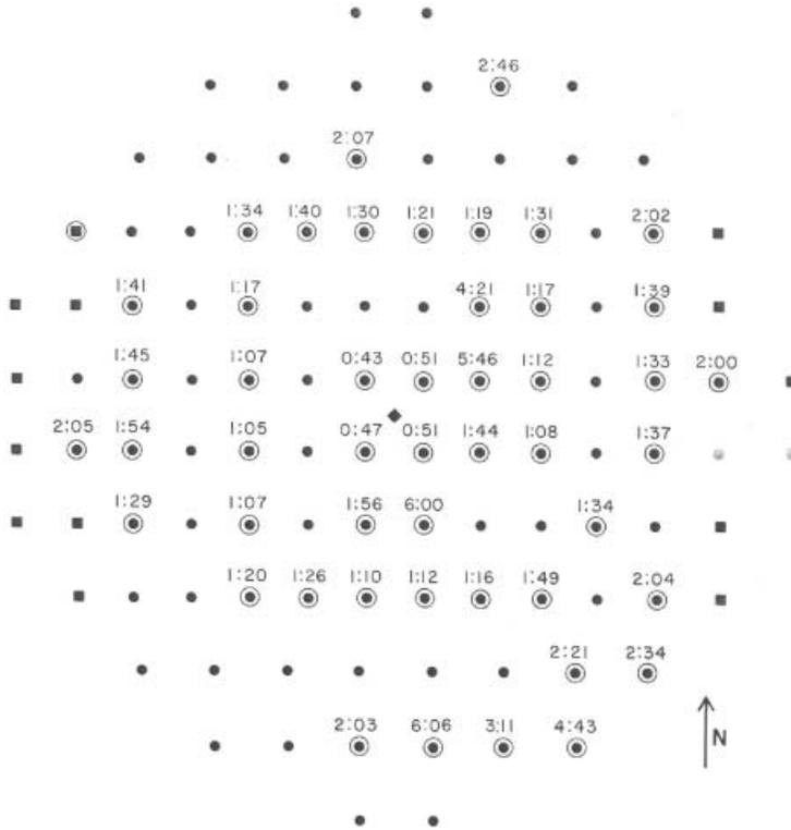
**Figure 8.** Sprinkler operating sequence of Test 2. • – timed sprinklers; ■ – nontimed sprinklers; ⊙ – operated sprinklers; ◆ – fire center.
