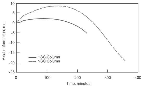
**Figure 2.** Axial deformation for the HSC and NSC columns.
