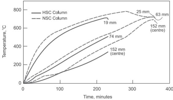
**Figure 1.** Temperature distribution at various depths in the NSC and HSC columns.
