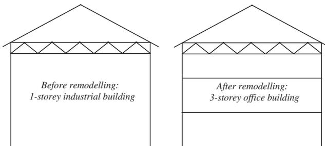
**Figure 3.** Layout before and after the remodelling of the industrial building.
