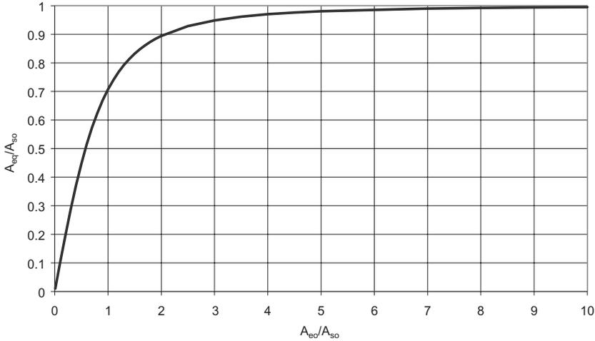
**Figure 3.** Equivalent opening area ratios.
