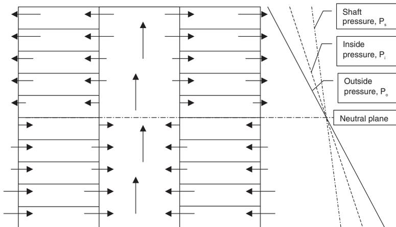
**Figure 4.** Schematic diagram of pressures and flow patterns during normal stack effect.
