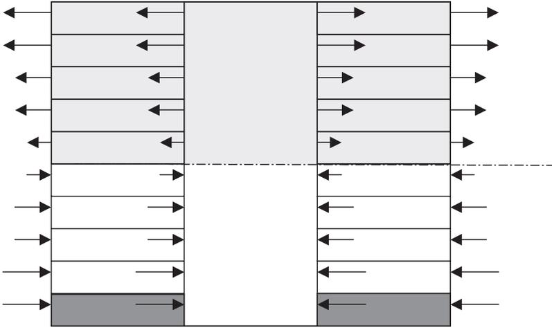
**Figure 9.** Qualitative steady-state conditions resulting from fire on first floor due to stack effect.
