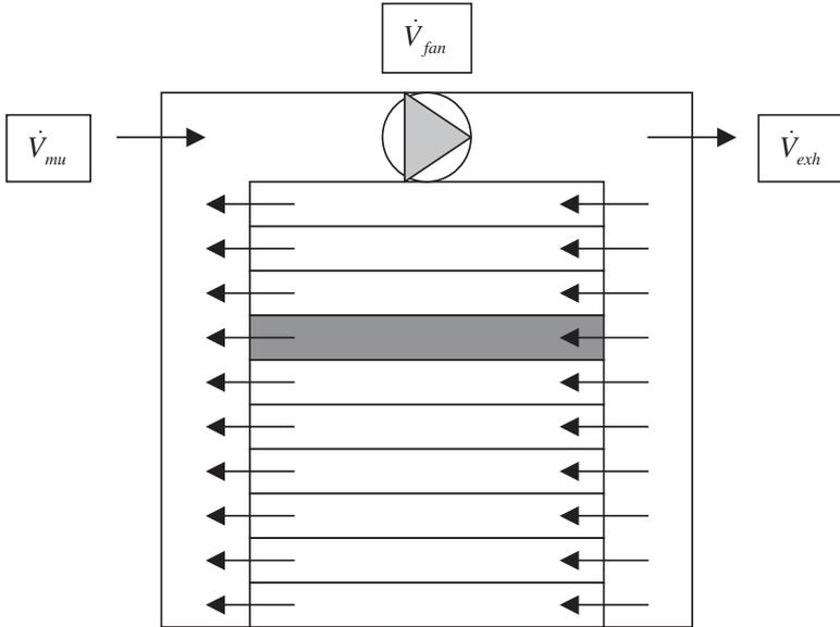
**Figure 18.** Schematic diagram of representative mechanical ventilation system.
