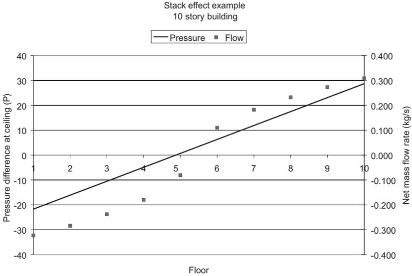
**Figure 7.** Stack effect example calculation for a 10-story building.
