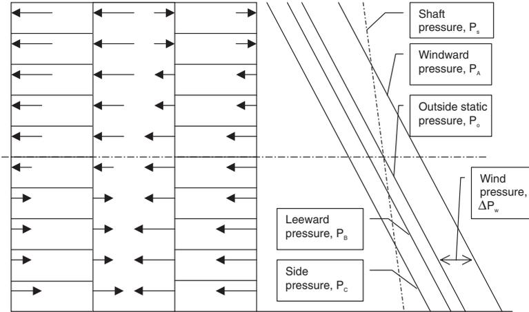
**Figure 11.** Schematic diagram of pressure differentials and flow patterns resulting from combination of stack and wind effects.
