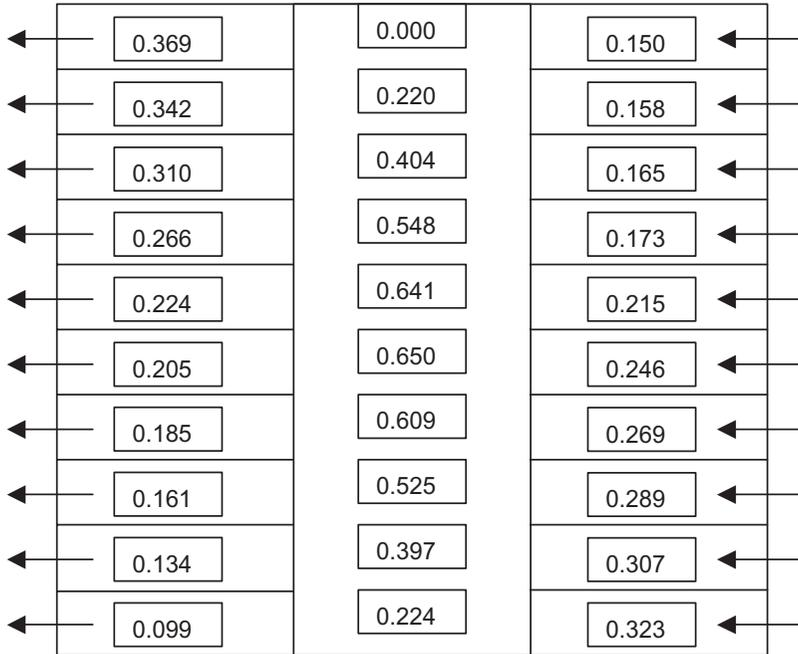
Figure 13. Schematic of mass flows in 10-story example building with wind effects.
