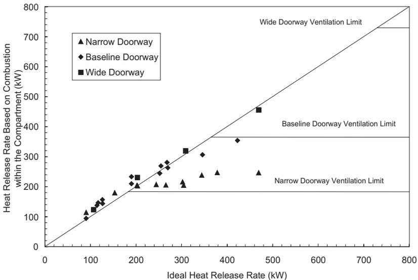
**Figure 6.** Heat release rate within compartment vs. ideal heat release rate.
