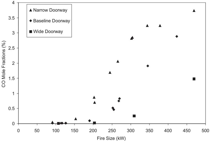
**Figure 5.** Carbon monoxide mole fractions as a function of the ideal fire size and doorway width.
