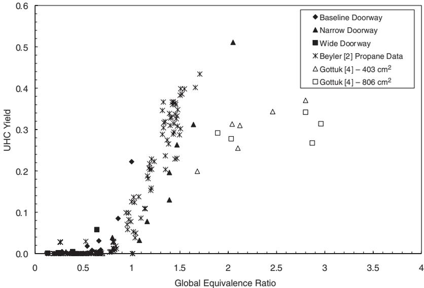
**Figure 4.** Unburned hydrocarbon yields as a function of the equivalence ratio and door width compared with data from [2,4].
