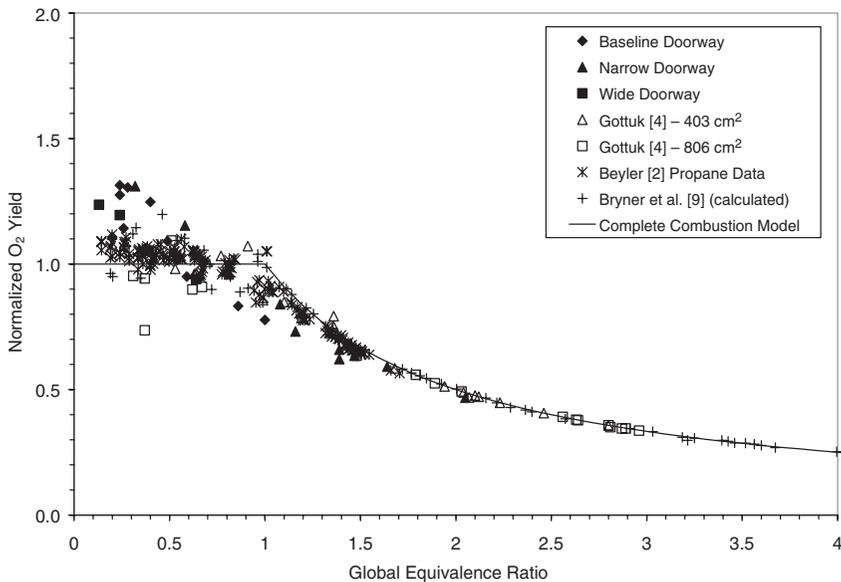
**Figure 1.** Normalized  $O_2$  yields as a function of the equivalence ratio and door width compared with data from [2,4,10] in addition to the model for complete combustion.
