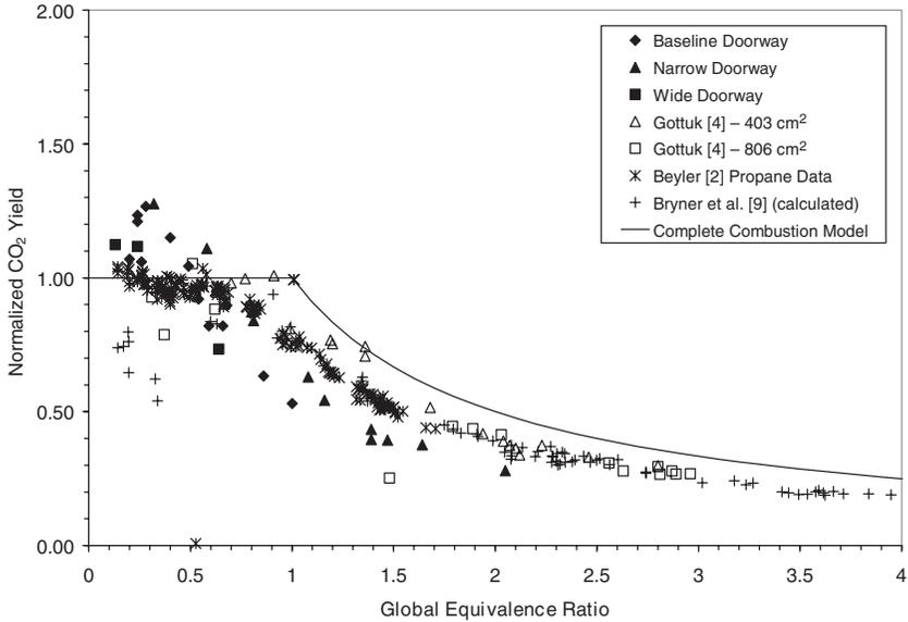
**Figure 2.** Normalized CO<sub>2</sub> yields as a function of the equivalence ratio and door width compared with data from [2,4,10] in addition to the model for complete combustion.
