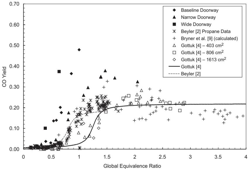
**Figure 3.** Carbon monoxide yields as a function of the equivalence ratio and door width compared with data from [2,4,10] in addition to models from [2,4].
