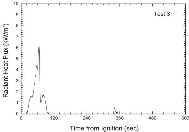
Figure 17. Radiant heat flux 1.2 m (4 ft) from the storage array measured in Test 3.
