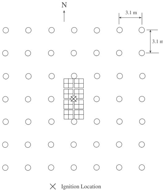
Figure 9. A plan view of the sprinkler layout relative to the storage array used in Test 4. The test was conducted under a 10.7-m (35 ft) high ceiling. The branch lines were in the east-west direction.
