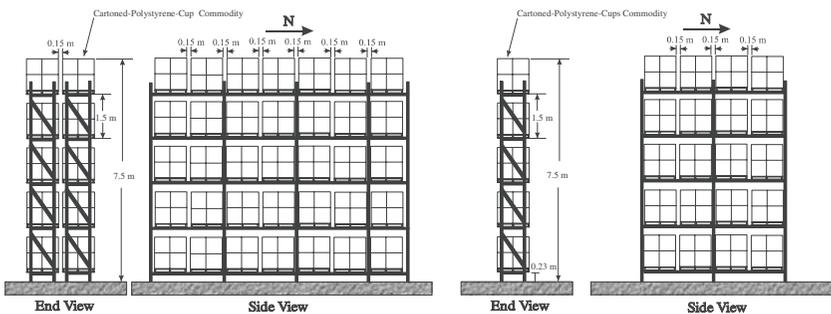
**Figure 2.** An illustration of the main storage array (on the left) and the target array (on the right) used in Test 1.
