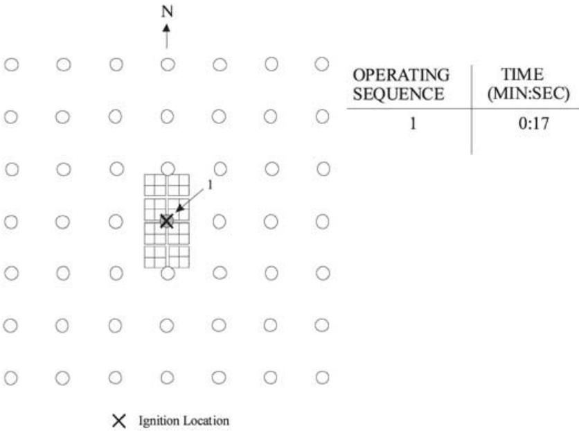
**Figure 19.** Actuated sprinklers (colored in gray) in Test 4.
