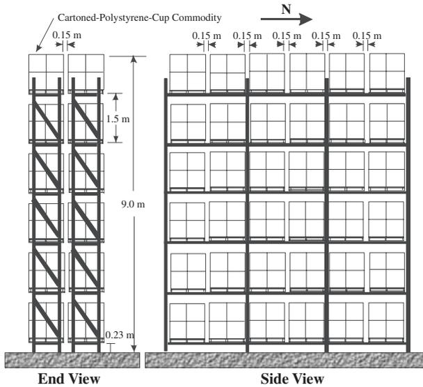
**Figure 10.** An illustration of the storage array used in Test 5.
