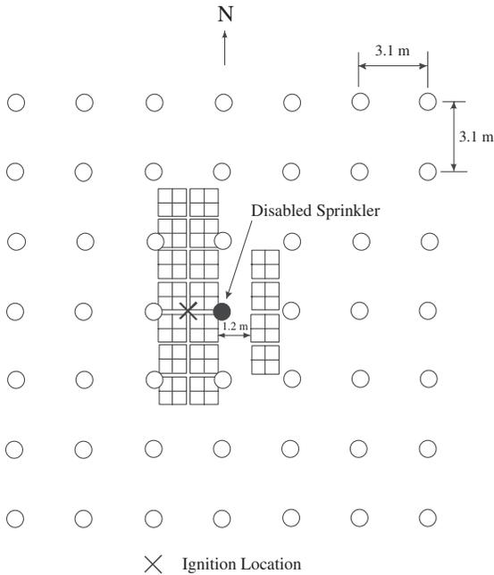
**Figure 3.** A plan view of the sprinkler layout relative to the storage arrays used in Test 1. The test was conducted under a 9.1-m (30 ft) high ceiling. The branch lines were in the east-west direction.
