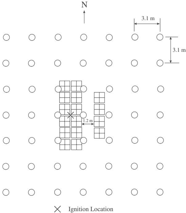
**Figure 4.** A plan view of the sprinkler layout relative to the storage arrays used in Test 2. The test was conducted under a 9.1-m (30 ft) high ceiling. The branch lines were in the east-west direction.
