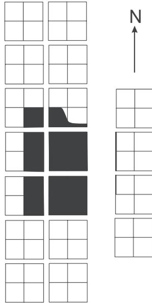
Figure 13. Extent of fire damage (colored in black) in Test 1.
