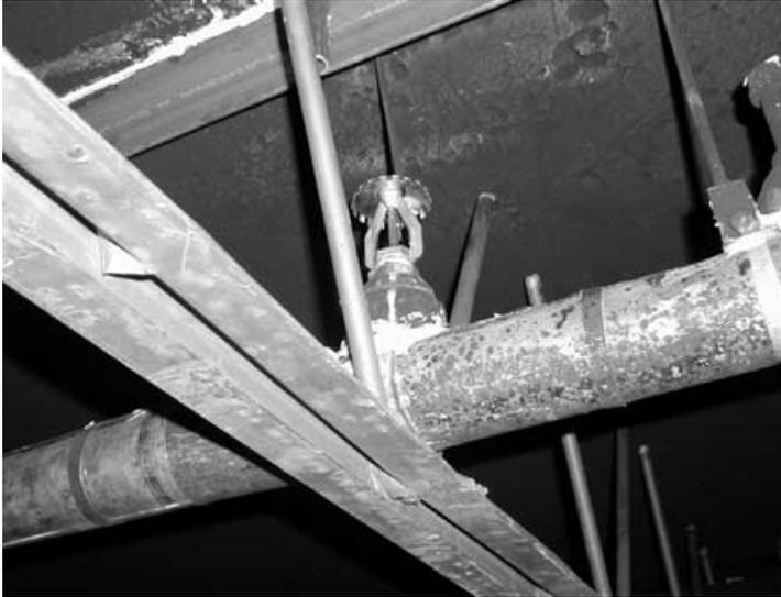
**Figure 7.** A photograph of the bar joist obstruction used in Test 3.
