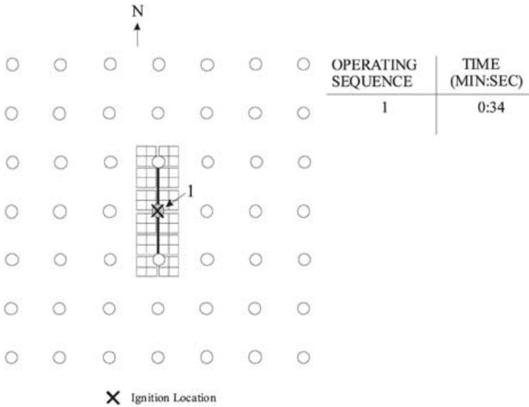
Figure 16. Actuated sprinklers (colored in gray) in Test 3.
