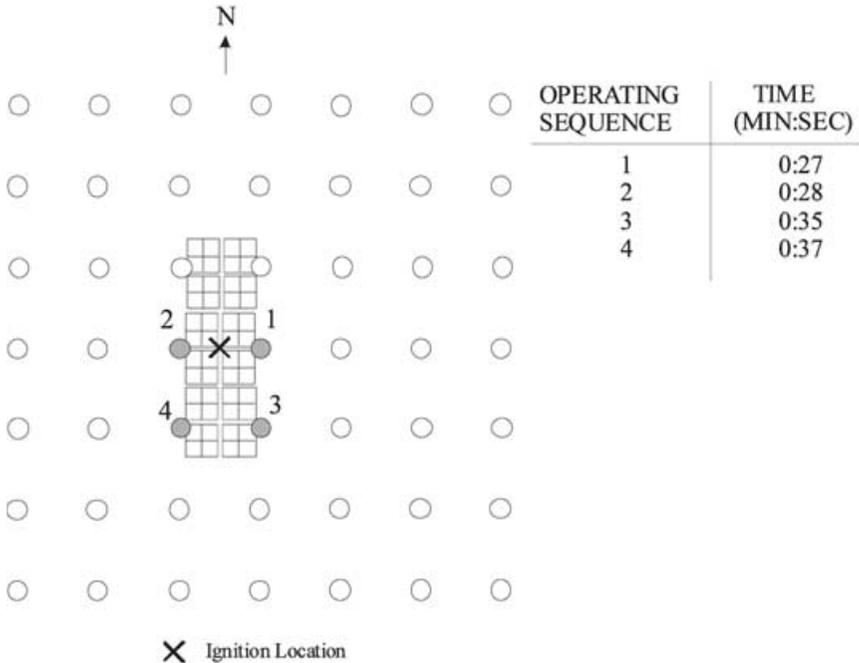
**Figure 22.** Actuated sprinklers (colored in gray) in Test 5.
