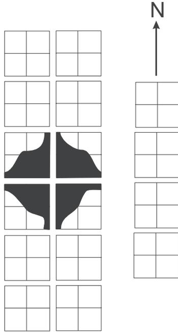
**Figure 15.** Extent of fire damage (colored in black) in Test 2.
