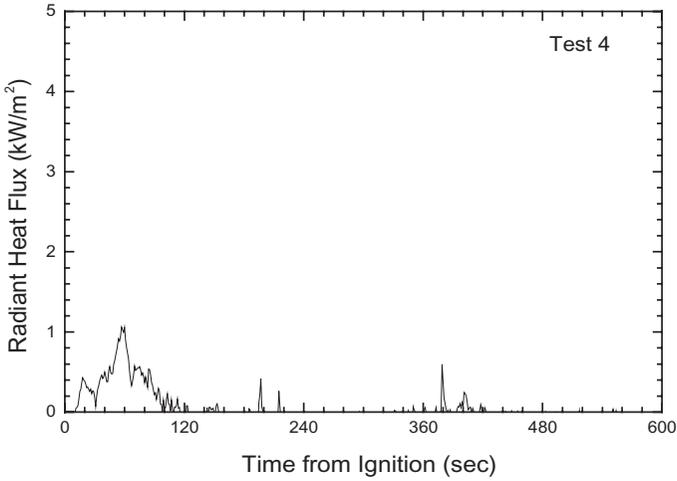
Figure 20. Radiant heat flux 1.2 m (4 ft) from the storage array measured in Test 4.
