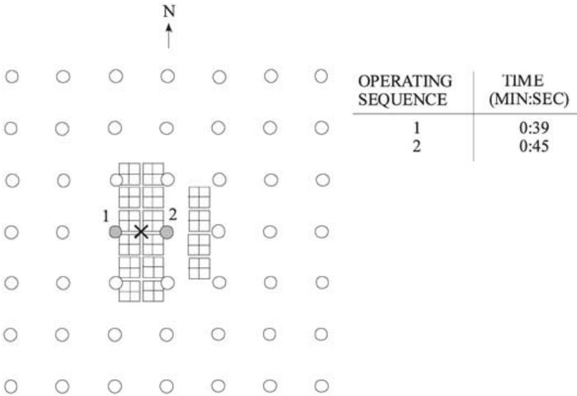
Figure 14. Actuated sprinklers (colored in gray) in Test 2.
