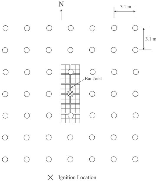
**Figure 6.** A plan view of the sprinkler layout relative to the storage array used in Test 3. The test was conducted under a 9.1-m (30 ft) high ceiling. The branch lines were in the east-west direction.
