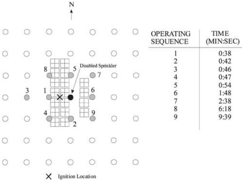
**Figure 12.** Actuated sprinklers (colored in gray) in Test 1.
