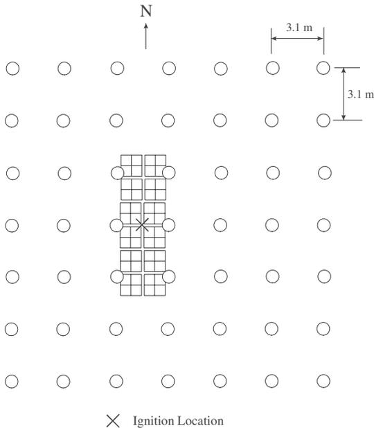
**Figure 11.** A plan view of the sprinkler layout relative to the storage array used in Test 5. The test was conducted under a 10.7-m (35 ft) high ceiling. The branch lines were in the east-west direction.
