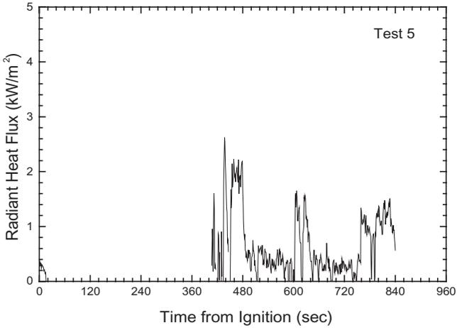
**Figure 23.** Radiant heat flux 1.2m (4ft) from the storage array measured in Test 5.
