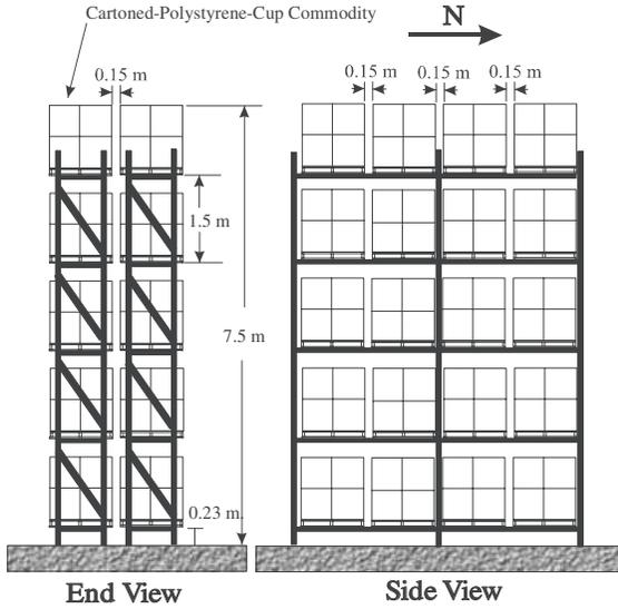
Figure 8. An illustration of the storage array used in Test 4.
