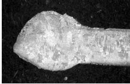
Figure 2. Bead created by experimental arcing – cross-section view (Courtesy Yasuaki Hagimoto).
