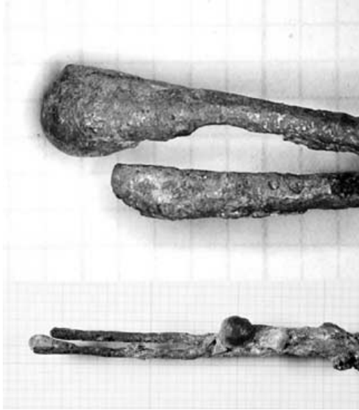
Figure 5. Examples of melted copper wire beads caused by exposure to fire without arcing (Courtesy Yasuaki Hagimoto).
