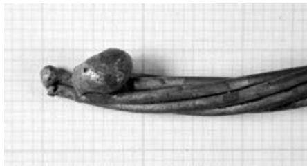
Figure 3. 'Victim' bead from a real fire (Courtesy Yasuaki Hagimoto).
