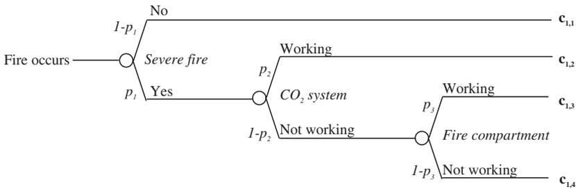
**Figure 3.** Event tree representing the possible consequences of a fire in the electrical equipment room, given that alternative 1 is chosen.
