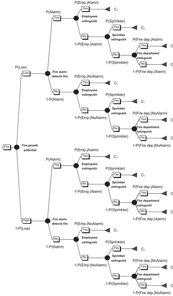
**Figure 6.** Event tree showing the different fire scenarios considered in the analysis of whether to invest in a sprinkler system.
