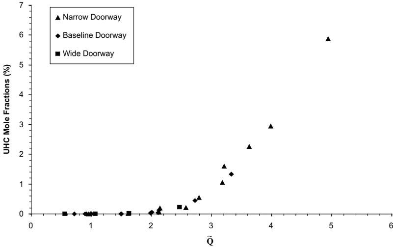
**Figure 12.** Integrated average unburned hydrocarbon mole fractions as a function of the nondimensional heat release rate parameter,  $\bar{Q}$ .
