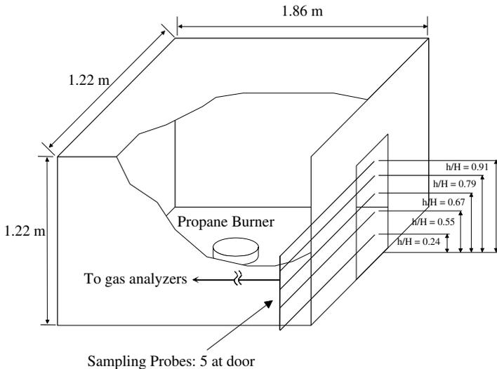
**Figure 2.** Half -scaled ISO 9705 compartment arrangement.
