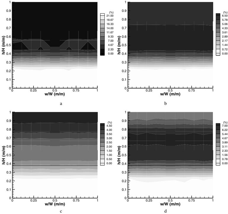
**Figure 7.** Narrow doorway species mapping of: (a)  $O_2$ ; (b)  $CO_2$ ; (c)  $CO$ ; and (d) UHC mole fractions (%), 470 kW (GER of 2.05), neutral plane determined from velocity probe data.
