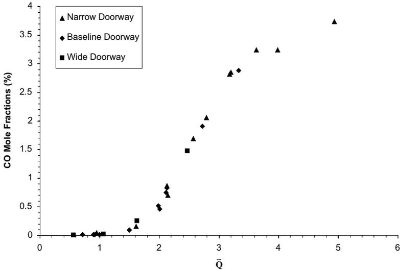
**Figure 11.** Integrated average carbon monoxide mole fractions as a function of the non-dimensional heat release rate parameter,  $\tilde{Q}$ .
