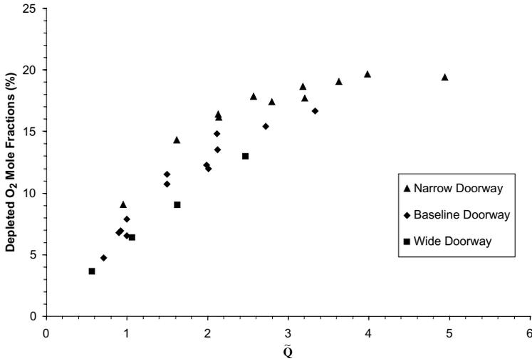
**Figure 9.** Integrated average oxygen mole fractions (depleted) as a function of the non-dimensional heat release rate parameter,  $\tilde{Q}$ .
