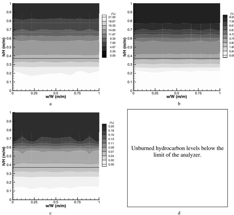
**Figure 4.** Narrow doorway species mapping of: (a)  $O_2$ ; (b)  $CO_2$ ; (c)  $CO$ ; and (d) UHC mole fractions (%), 153 kW (GER of 0.58), neutral plane determined from velocity probe data.
