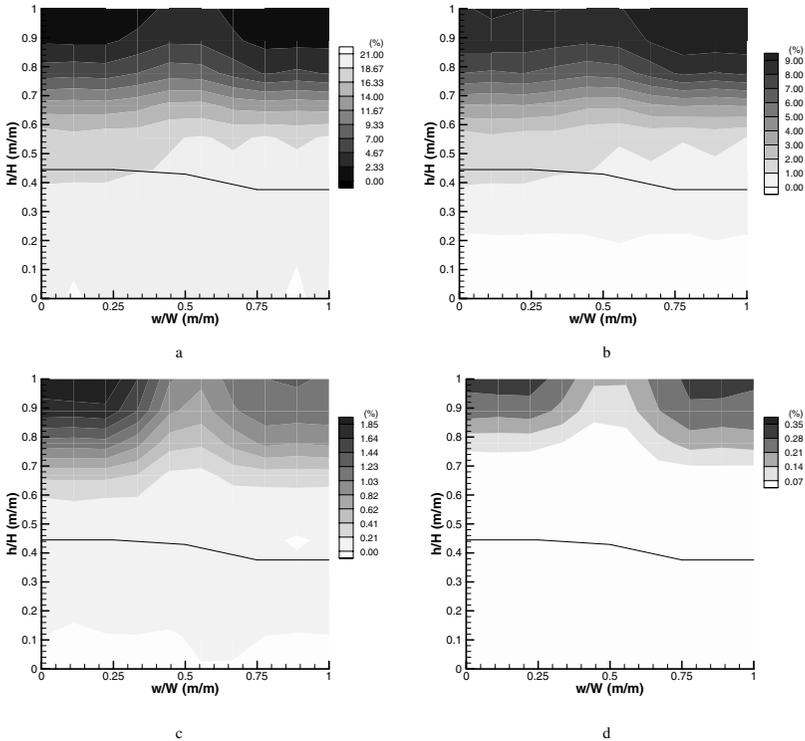
**Figure 5.** Baseline doorway species mapping of: (a)  $O_2$ ; (b)  $CO_2$ ; (c)  $CO$ ; and (d) UHC mole fractions (%), 270 kW (GER of 0.56), neutral plane determined from velocity probe data.
