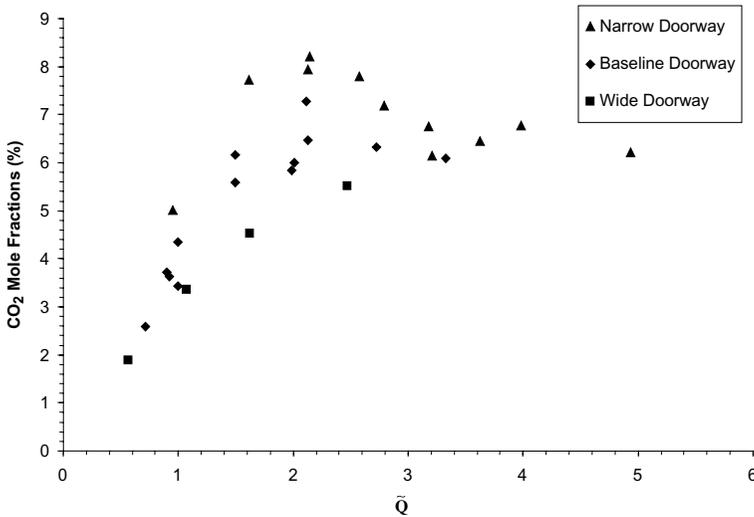
**Figure 10.** Integrated average carbon dioxide mole fractions as a function of the non-dimensional heat release rate parameter,  $\tilde{Q}$ .
