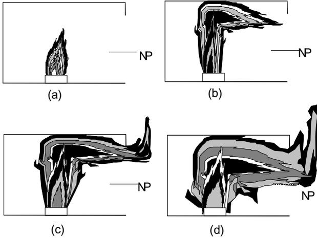
**Figure 8.** Illustration of four  $\tilde{Q}$  conditions: (a)  $\tilde{Q} < 1.0$ ; (b)  $\tilde{Q} = 1.0$ ; (c)  $1.0 < \tilde{Q} < \tilde{Q}_{critical}$ ; (d)  $\tilde{Q} > \tilde{Q}_{critical}$ . NP = Neutral plane elevation in the doorway.
