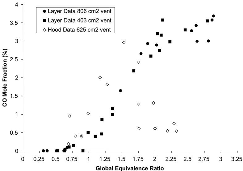
**Figure 1.** Comparison between carbon monoxide levels measured in the compartment upper layer and the exhaust hood by Gottuk [5].
