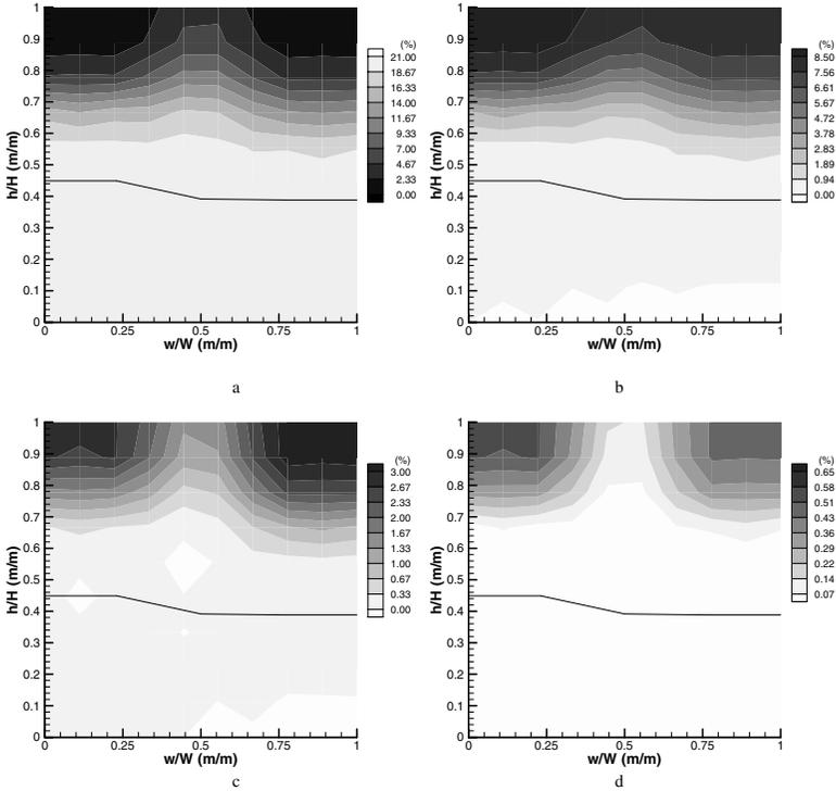
**Figure 6.** Wide doorway species mapping of: (a)  $O_2$ ; (b)  $CO_2$ ; (c)  $CO$ ; and (d) UHC mole fractions (%), 470 kW (GER of 0.64), neutral plane determined from velocity probe data.
