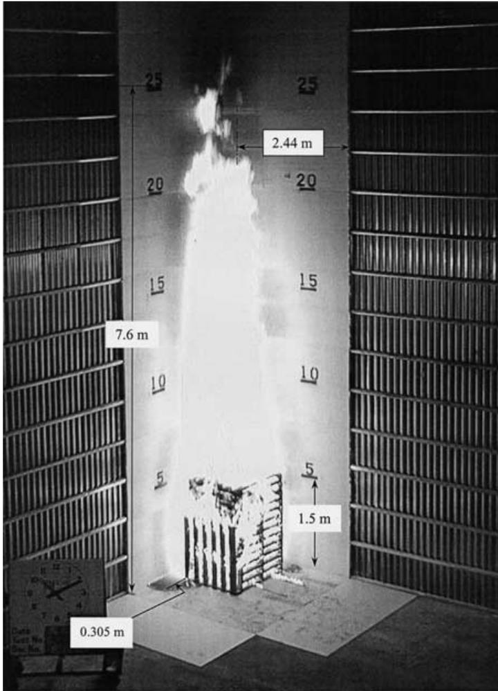
**Figure 2.** Photograph of Inert-Wall Test about 650s after ignition.
