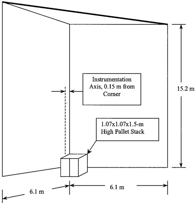
**Figure 1.** Schematic of 50-ft Corner Test facility.
