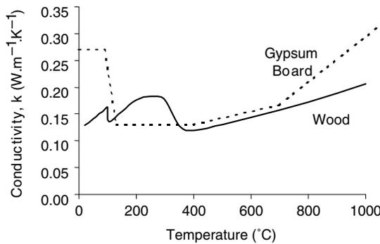
Figure A-3. Conductivities of gypsum board [33,14] and wood [25] with temperature.
