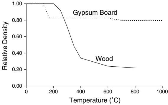
Figure A-1. Relative densities of gypsum board [33] and wood [25] with temperature.
