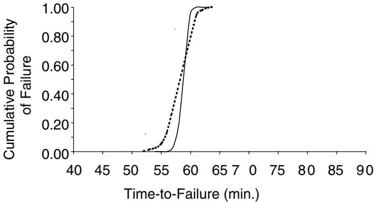
**Figure 9.** Cumulative probability of failure with time for wood-framed wall with controlled selection of studs: — CoV for specific heat and conductivity of timber = 0.02; - - - CoV for specific heat and conductivity of timber = 0.10.
