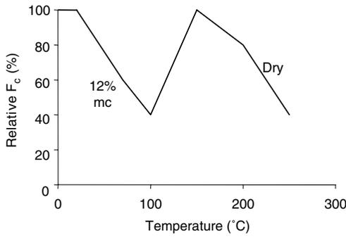
**Figure A-5.** Relative compression strength of timber vs. temperature [26].
