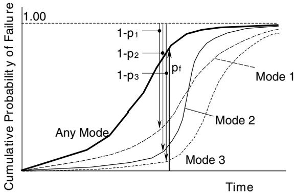
**Figure 6.** Total probability of failure from three modes of failure.
