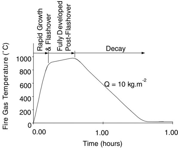
Figure 11. Real fire severity used in evaluation.
