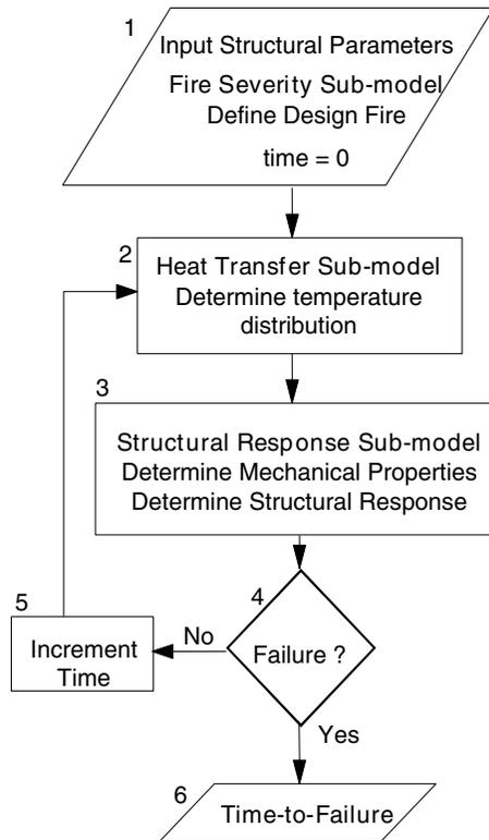
**Figure 1.** Time-to-failure model.
