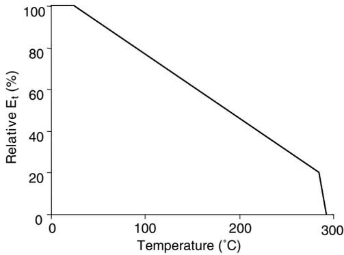
**Figure A-6.** Relative elastic modulus of timber in tension vs. temperature [21].
