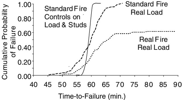
Figure 12. Comparison of the cumulative probabilities of failure with a realistic variation in mechanical properties and loads, subjected to real fire.
