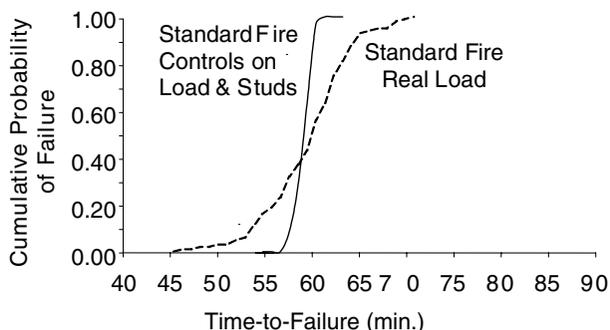
**Figure 10.** Comparison of the cumulative probabilities of failure with time for wood-framed wall with a realistic variation in mechanical properties and loads, subjected to standard fire [16].
