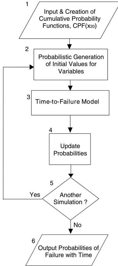
Figure 2. Probability of failure with time model.
