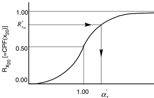
**Figure 5.** Generation of independent random parameter,  $\alpha'_x$ , from random number,  $R^*_{x_{20}}$ , and cumulative probability of failure function,  $CPF(x_{20})$ .
