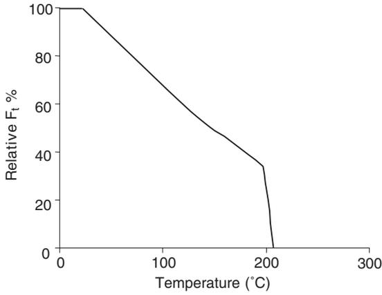
**Figure A-4.** Relative tensile strength of timber vs. temperature [12].
