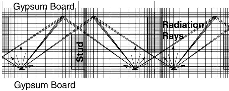
**Figure 3.** Examples of rays considered in a discrete radiative heat transfer analysis for a staggered stud wall.
