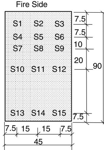
**Figure 7.** Positions of thermocouples S1–S15 in studs; all dimensions in mm.
