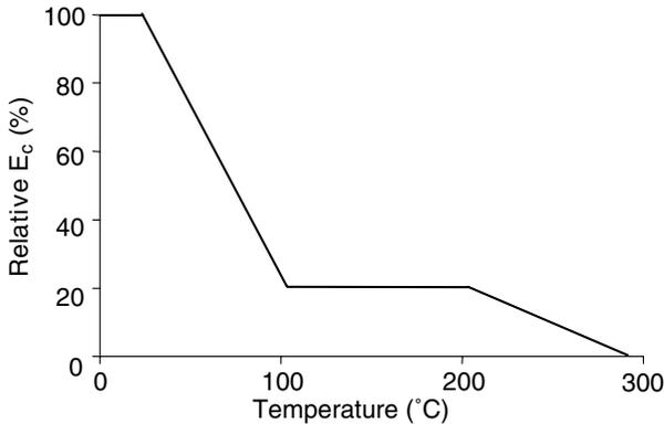
**Figure A-7.** Relative elastic modulus of timber in compression vs. temperature [26].
