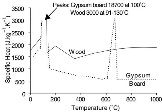
Figure A-2. Specific heats of gypsum board [34] and wood [25] with temperature.
