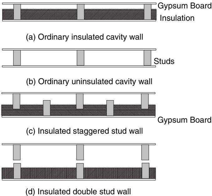
**Figure 4.** Range of light timber framed wall sections.
