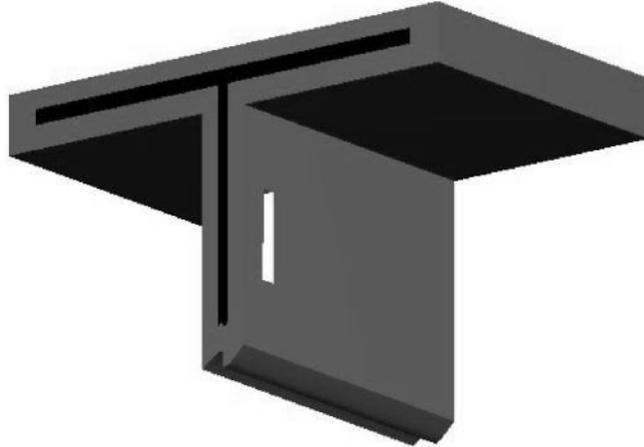
Figure 4. Diagram of half of steel column with missing protection on web.
