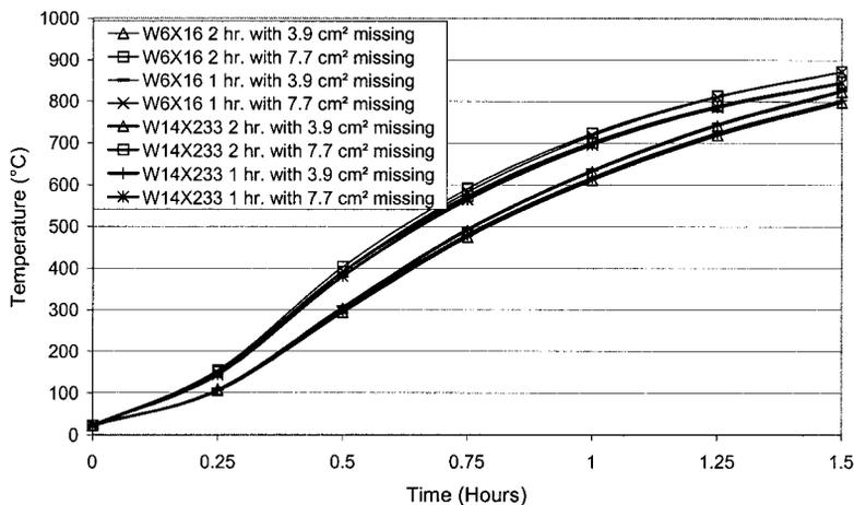
**Figure 9.** Comparison of temperatures at exposed flange surface.
