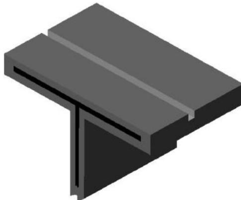
**Figure 3.** Diagram of half of steel column with missing protection on flange.
