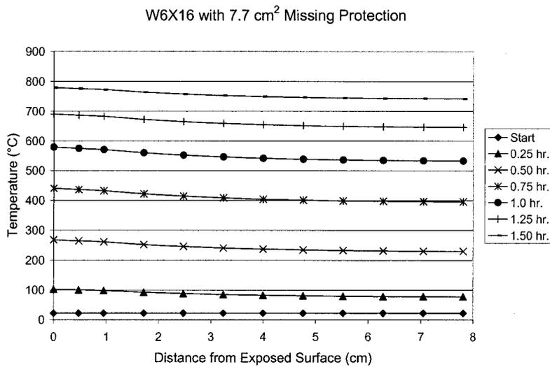
Figure 5. Temperature profile perpendicular to the flange.
