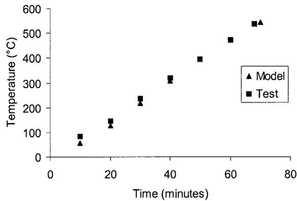
**Figure 2.** Average temperature of W10 × 49 steel column with 19 mm of protection.
