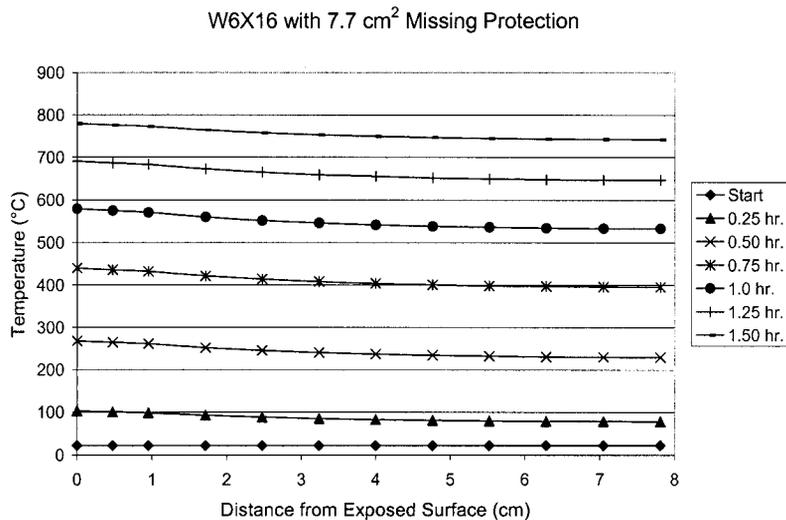
Figure 6. Temperature profile over the column length.
