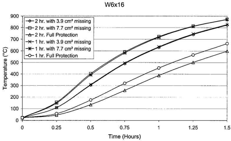
Figure 7. Temperature at exposed flange surface.
