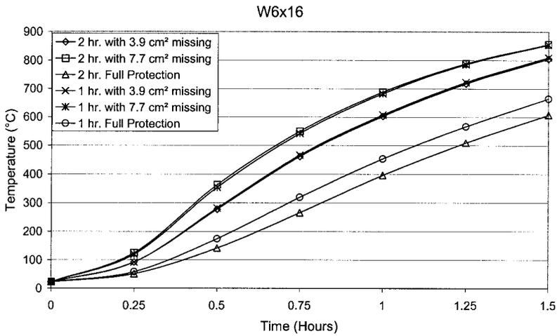
Figure 8. Temperature at exposed web surface.
