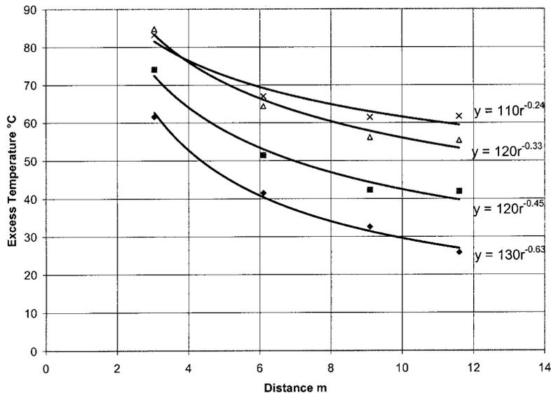
**Figure 3.** Time evolution of the radial temperature dependence of the ceiling jet for the 7.7 MW JP-5 pan fire with draft curtain at a 15 m high ceiling. The four curves correspond to experimental times of 70 s, 100 s, 200 s, and 300 s from bottom to top respectively.
