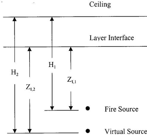
**Figure 1.** Graphical representation of the relationship between the fire source ( $Q_{I,1}$ ) and the virtual source ( $Q_{I,2}$ ).
