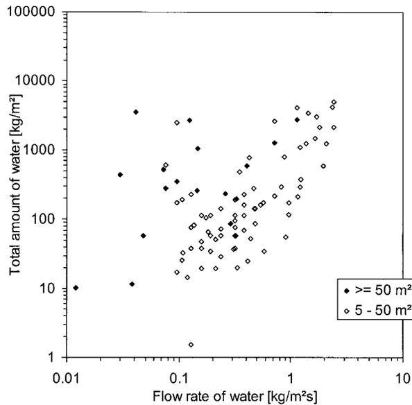
**Figure 7.** The total volume of water versus the flow rate, in real fires.
