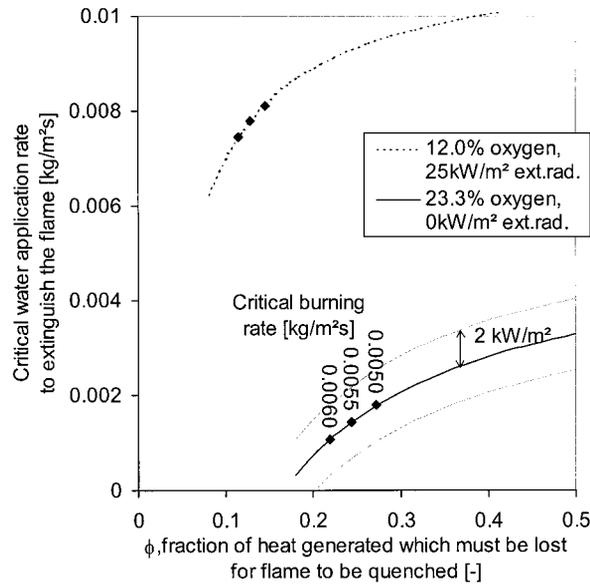
**Figure 1.** Relation between the critical water application rate and the fraction of heat which must be lost for the flame to be quenched. The solid line represents well-ventilated conditions and the surrounding lines represent  $2 \text{ kW/m}^2$  heat added or removed. The dotted line represents under-ventilated conditions with high external radiation due to a flashover fire.
