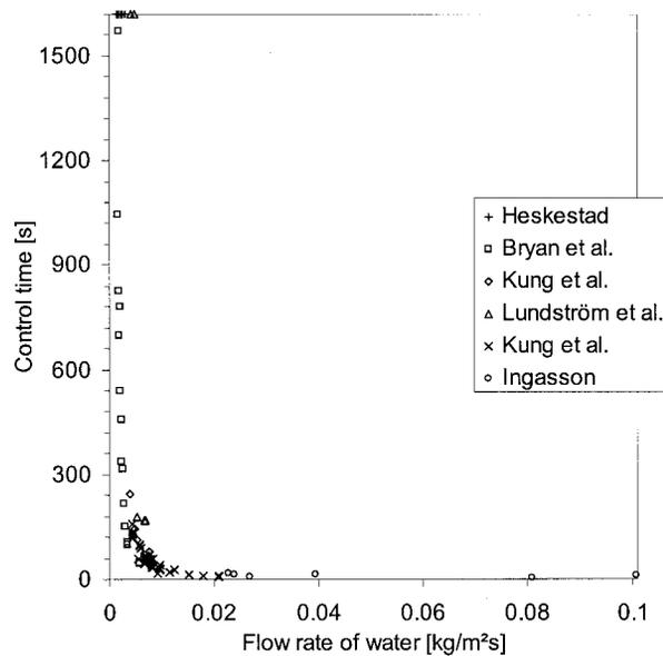
**Figure 5.** The control time as a function of the flow rate. Note that the Lundström tests were performed with near-flashover room temperatures.
