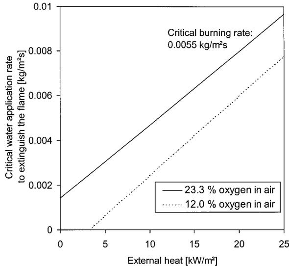
**Figure 2.** External heat versus the critical water application rate.
