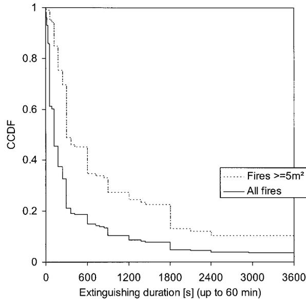
**Figure 8.** The complementary cumulative distribution function of the extinction duration for all the real fires investigated and when fires larger than  $5\text{ m}^2$  were selected.
