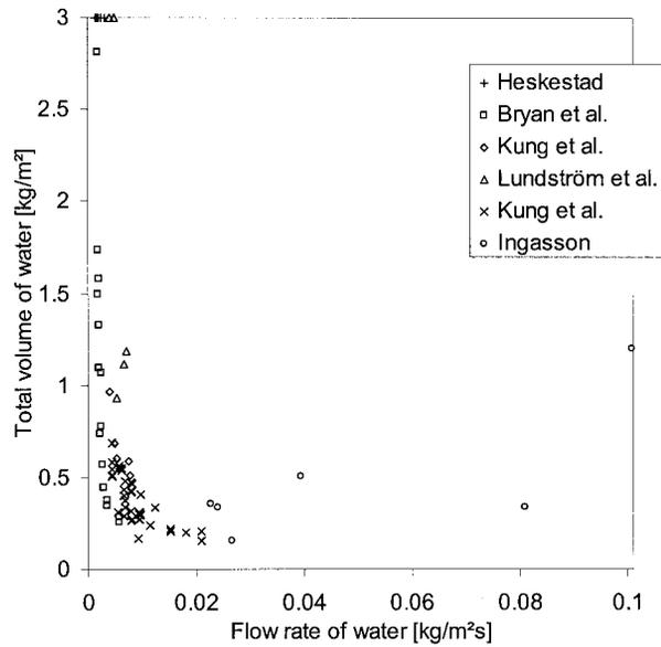
**Figure 4.** The total amount of water used as a function of the flow rate. Note that the high room temperature in the Lundström tests increased the water demand.
