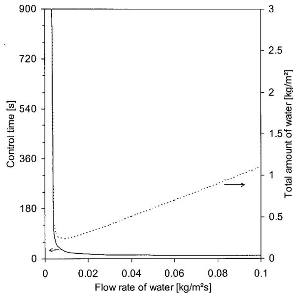
**Figure 3.** The control time (solid) and the total amount of water (dotted) as a function of the water flow rate.
