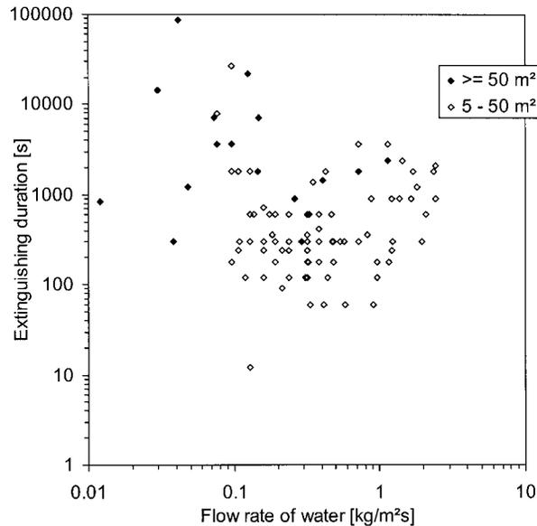
**Figure 6.** The duration of the attack as a function of the flow rate. Filled marks represent fires with a horizontal fire area larger than  $50 \text{ m}^2$ .
