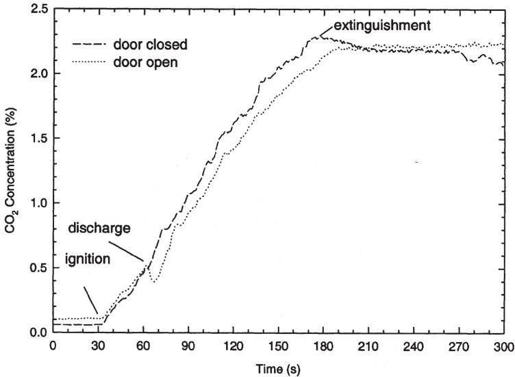
**Figure 17.** CO<sub>2</sub> concentrations in the compartment with the door closed and open for the pool fire tests, when the twin-fluid/low pressure water mist system was employed.
