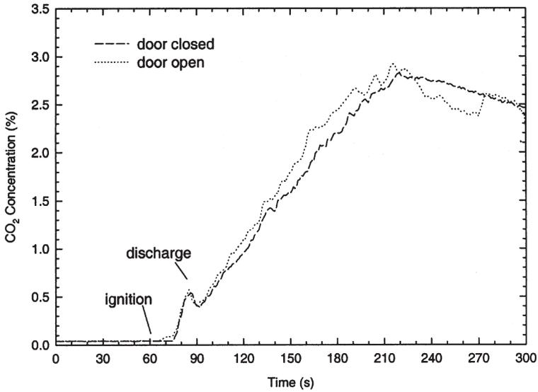
**Figure 14.** CO<sub>2</sub> concentrations in the compartment with the door closed and open in the spray fire test, when the single-fluid/high pressure water mist system was employed.
