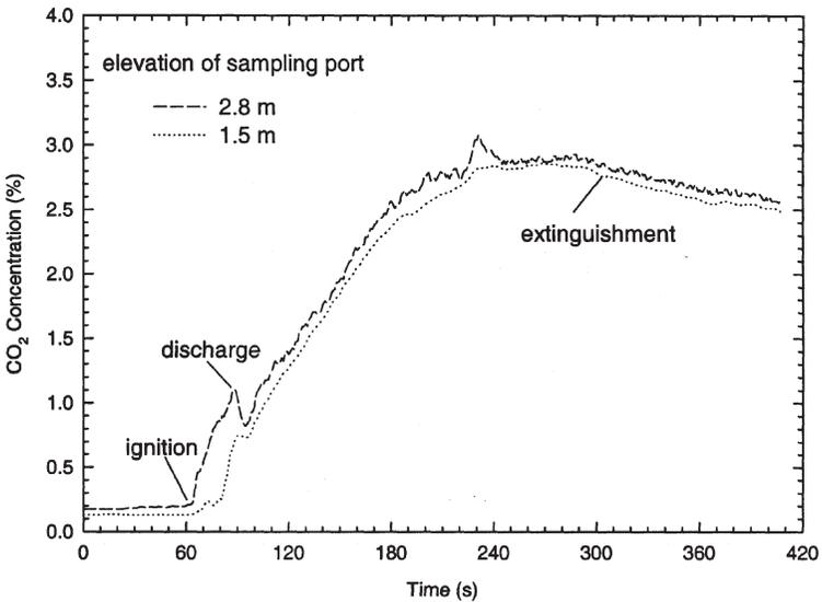
**Figure 6.** CO<sub>2</sub> concentrations in the compartment in Test 1-1 with pool fires, when the single-fluid/high pressure water mist system was employed and the door was closed.
