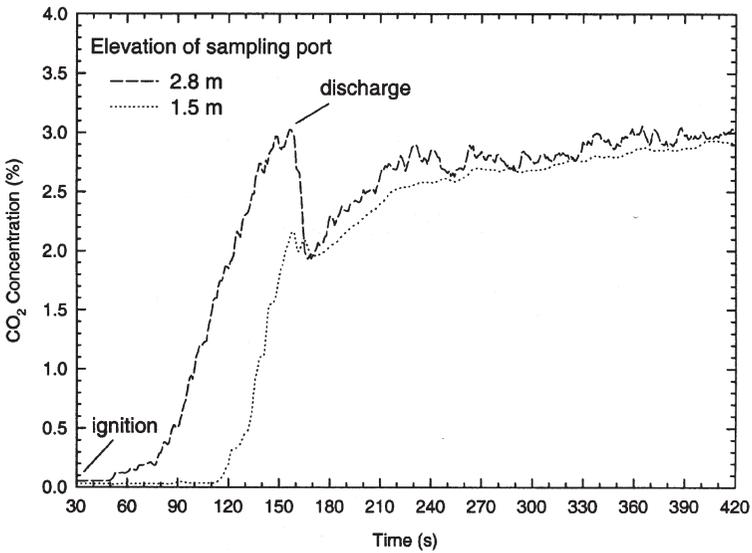
**Figure 8.** CO<sub>2</sub> concentrations in the compartment in Test 1-2 with wood crib fire, when the single-fluid/high pressure water mist system was employed and the door was closed.
