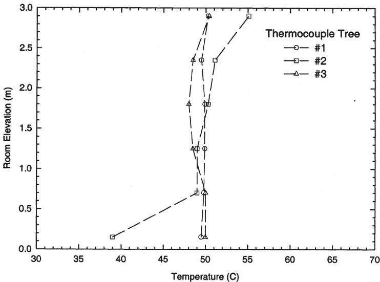
**Figure 16.** Room temperature profiles along the elevations measured at thermocouple trees when the door was open for the pool fire tests with twin-fluid/low pressure mist system at 90 s after mist discharge.
