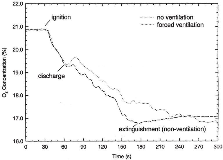
**Figure 19.** O<sub>2</sub> concentrations in the compartment in the spray fire tests with no ventilation and with forced ventilation, when a twin-fluid/low pressure water mist system was employed in the machinery space.
