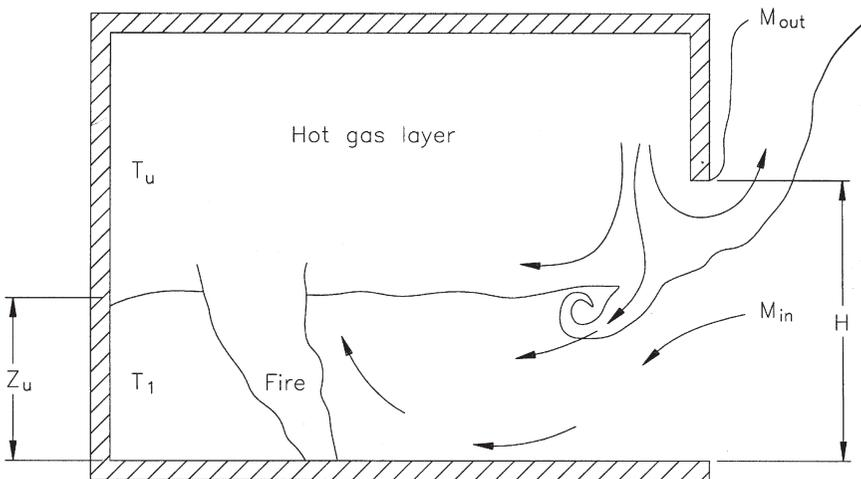
**Figure 9.** A schematic of convective mass transfer phenomena within a compartment.
