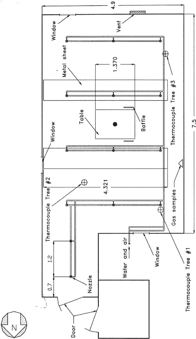
Figure 3. Test facilities, fire locations and a twin-fluid water mist system in engine mock-up test (plan).
