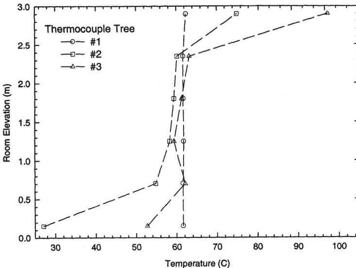
**Figure 18.** Room temperature profiles along the elevations measured at thermocouple trees under forced ventilation for the spray fire test with twin-fluid/low pressure mist system at 50 s of discharge.
