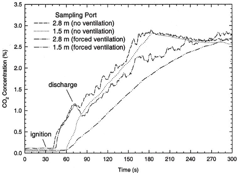
**Figure 20.** CO<sub>2</sub> concentrations in the compartment during the spray fire tests with no ventilation and with forced ventilation, when the twin-fluid/low pressure water mist system was employed.
