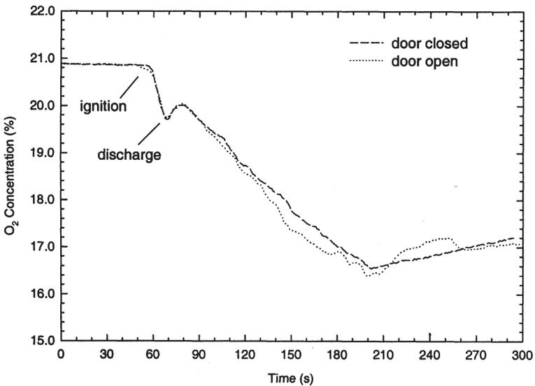
**Figure 15.** O<sub>2</sub> concentrations in the compartment with the door closed and open in the spray fire tests, when the single-fluid/high pressure water mist system was employed.
