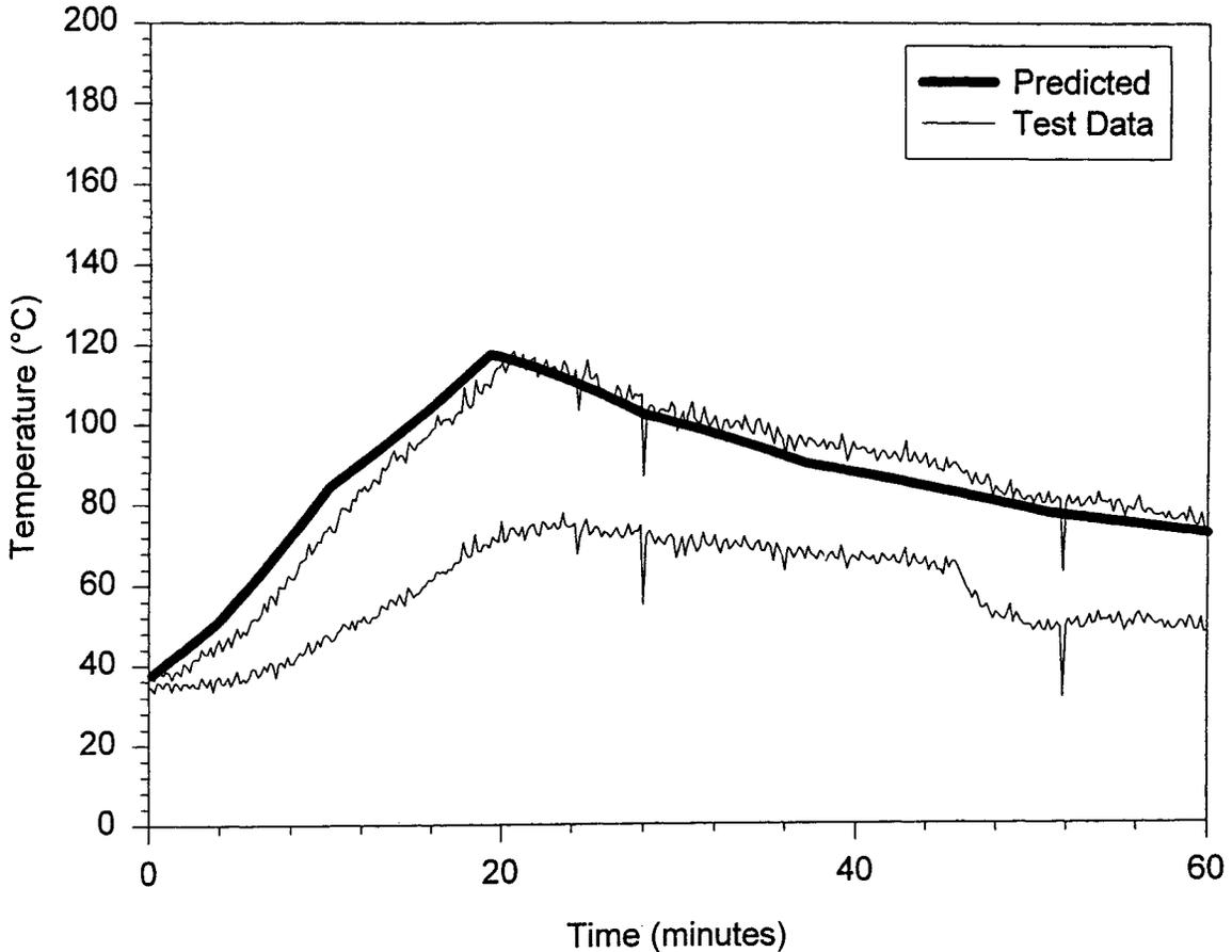
Figure 13. Gas temperatures for CPO Mess: predicted vs. full scale.
