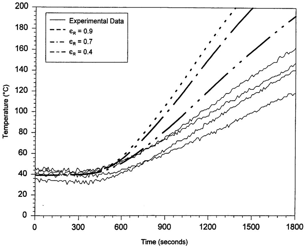
Figure 4. Comparison of modeled wall temperature vs. experimentally measured west wall temperatures: effects of resultant emissivity.
