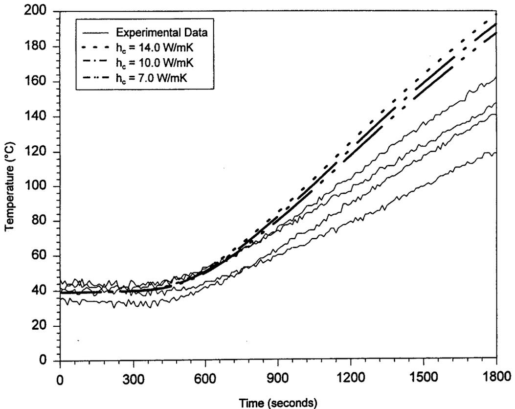
Figure 6. Comparison of modeled compartment wall temperature vs. experimentally measured west wall temperatures: effects of hot wall convection coefficient.
