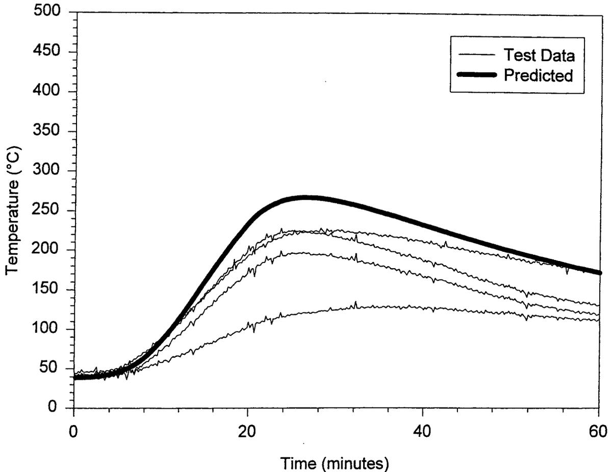
Figure 14. Bulkhead temperatures for RICER 2: predicted vs. full scale.
