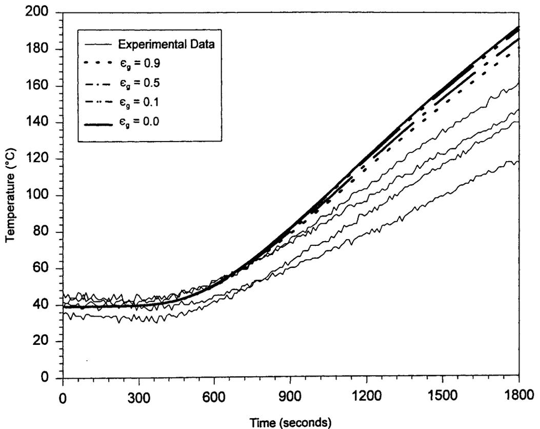
Figure 8. Comparison of modeled wall temperature vs. experimentally measured west wall temperatures: effects of gas emissivity.
