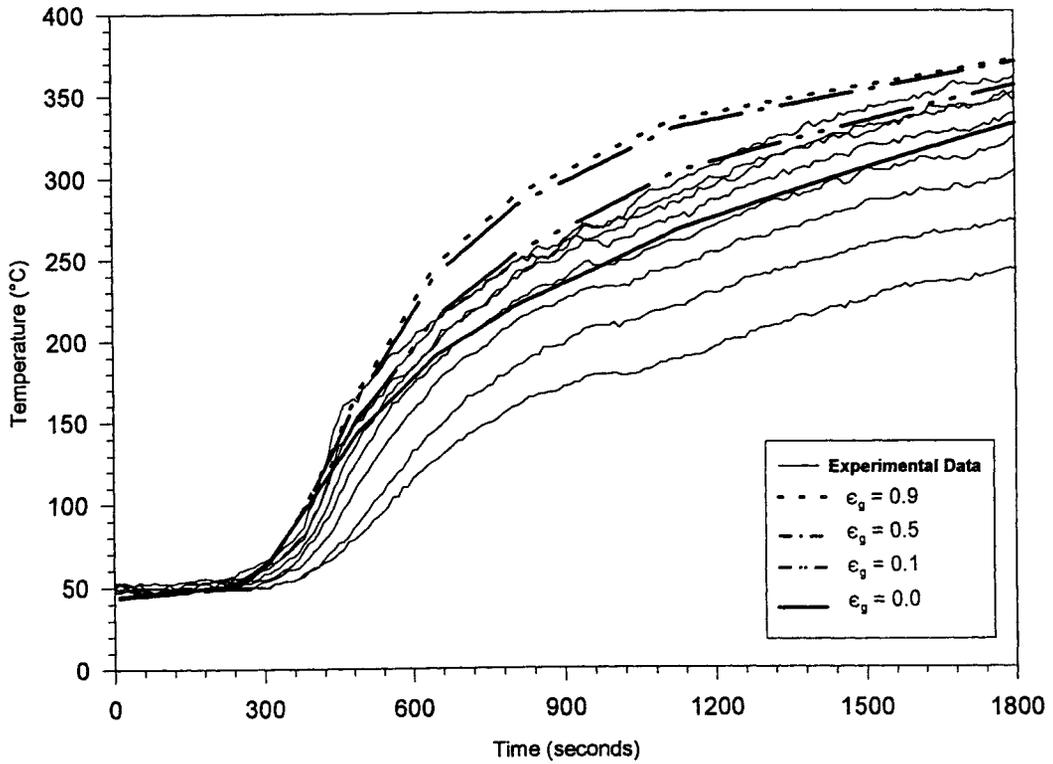
Figure 7. Comparison of modeled compartment gas temperature vs. experimentally measured west compartment gas temperatures: effects of gas emissivity.
