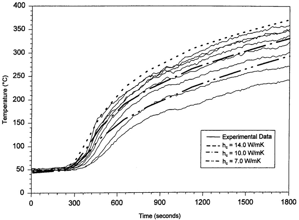
Figure 5. Comparison of modeled compartment gas temperature vs. experimentally measured west compartment gas temperatures: effects of hot wall convection coefficient.
