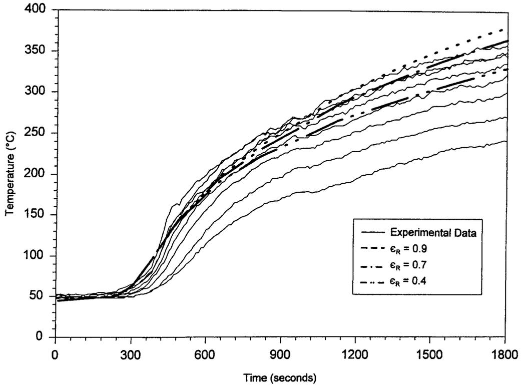
Figure 3. Comparison of modeled compartment gas temperature vs. experimentally measured west compartment gas temperatures: effects of resultant emissivity.
