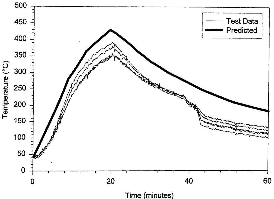
Figure 12. Gas temperatures for RICER 2: predicted vs. full scale.
