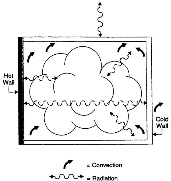
Figure 1. Modes of heat transfer modeled.
