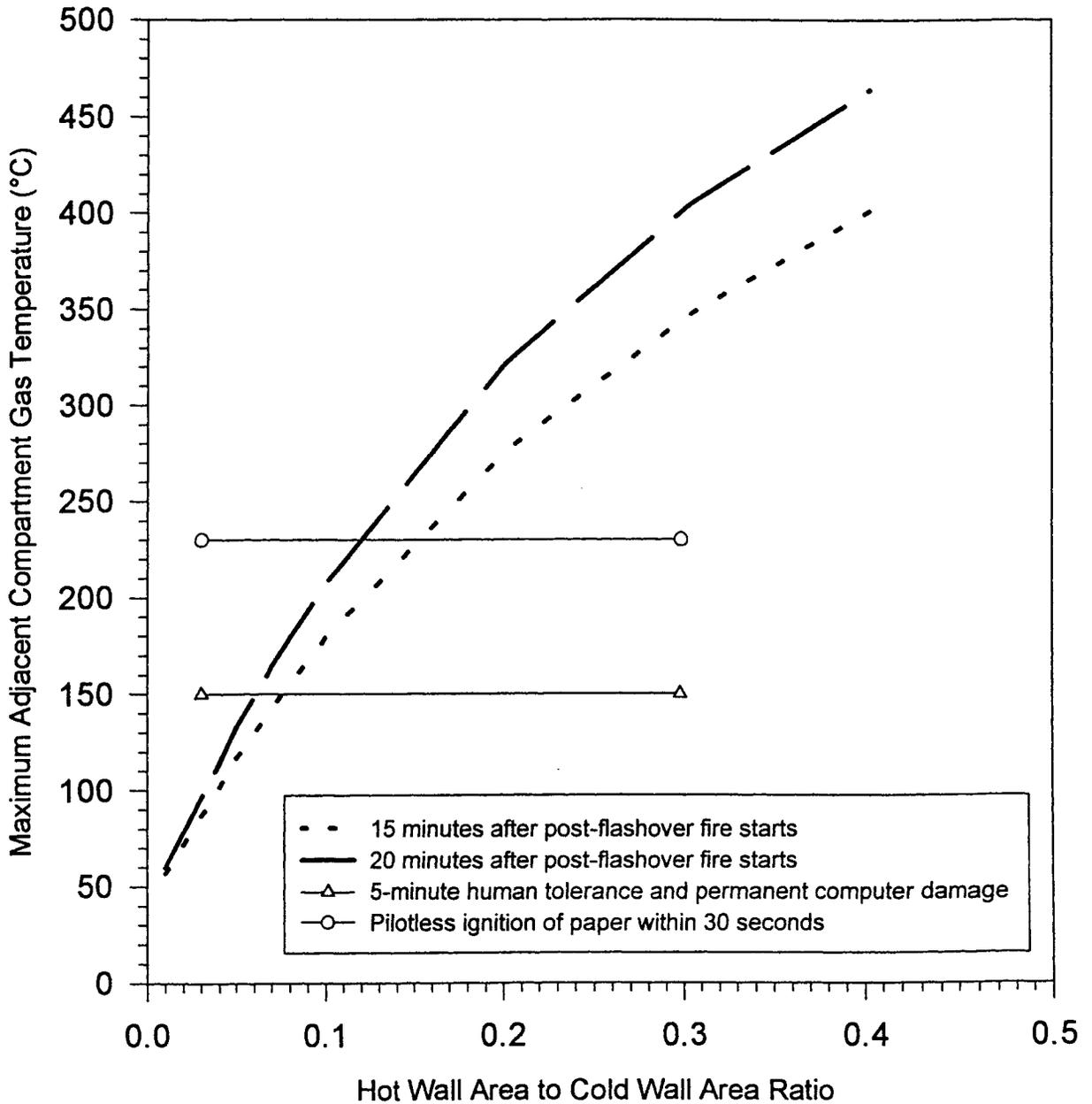
Figure 15. Relationship between hot wall and cold wall area ratio and thermal effects in adjacent compartments.
