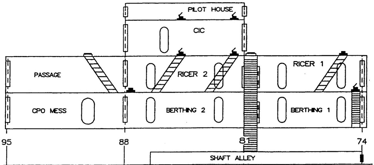
Figure 9. Compartment arrangement for full-scale tests.
