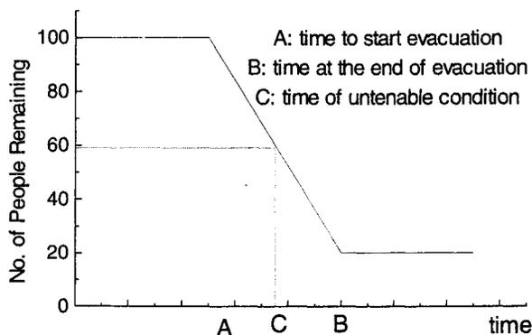
Figure 1. Hasofer's Linear Evacuation Example
